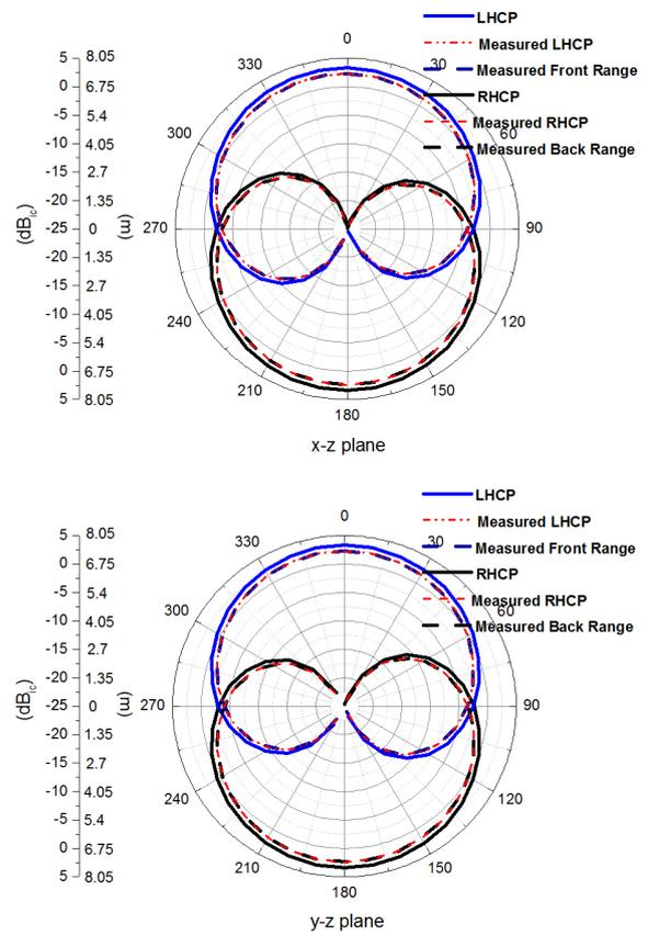
Fig. 9. Simulated and measured radiation pattern along with measured range.
