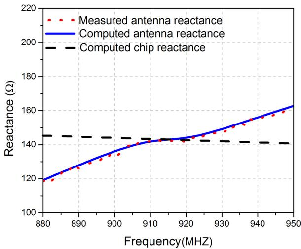
Fig. 6. Computed and measured reactance of the tag antenna.
