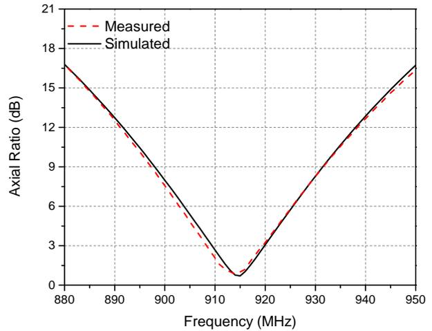
Fig. 8. Simulated and measured axial ratio of CP tag antenna.
