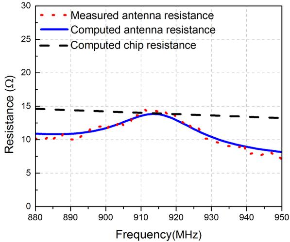
Fig. 5. Computed and measured resistance of the tag antenna.
