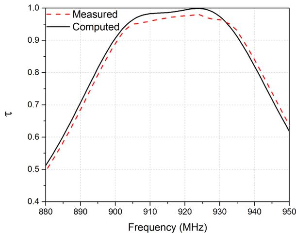
Fig. 7. Computed and measured power transmission coefficient of the tag antenna.
