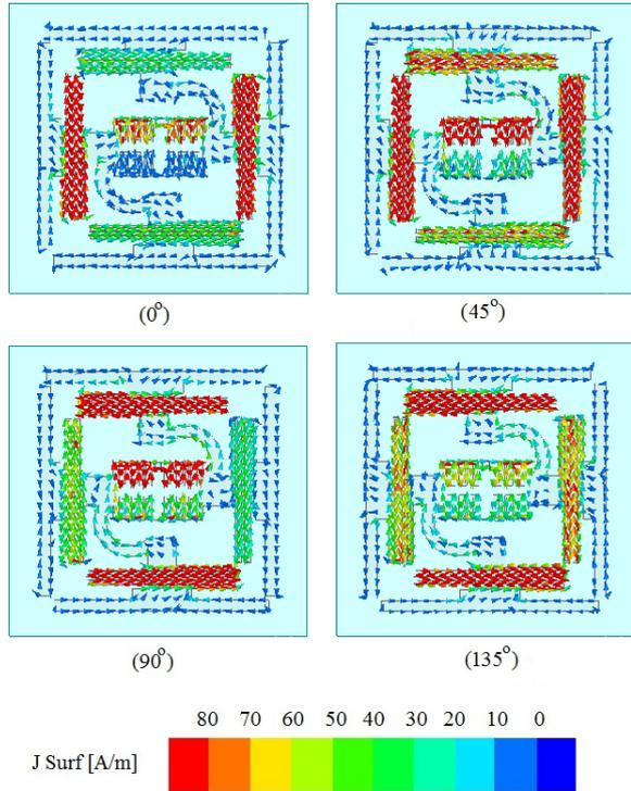
Fig. 3. Simulated current distribution of RFID tag at 915 MHz for two phases.
