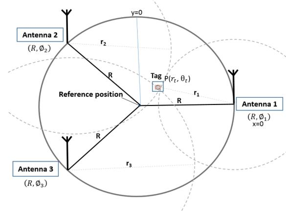
**Fig. 11.** Reader antenna's and tag positions in the interrogation region.
