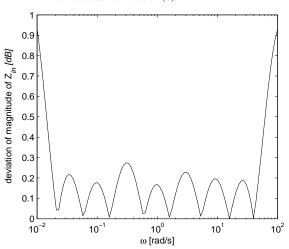
Fig. 9. Magnitude deviation of  $Z_{in}$  of the synthesized circuit.
