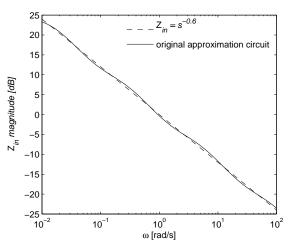
Fig. 3. Comparison of magnitude of  $Z_{in}$  of the original approximation circuit and ideal function (6).
