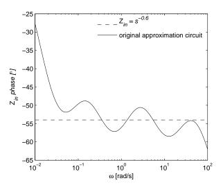
**Fig. 5.** Comparison of phase of  $Z_{in}$  of the original approximation circuit and ideal function (6).
