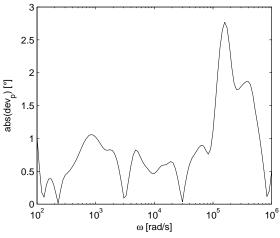
Fig. 18. Phase deviation of the measured circuit.
