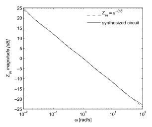
**Fig. 8.** Comparison of magnitude of  $Z_{in}$  of the synthesized circuit and desired function (6).
