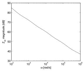
**Fig. 13.** Magnitude characteristic of  $Z_{in}$  of the transformed circuit
