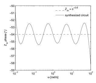
Fig. 10. Comparison of phase of  $Z_{in}$  of the synthesized circuit and the desired function (6).
