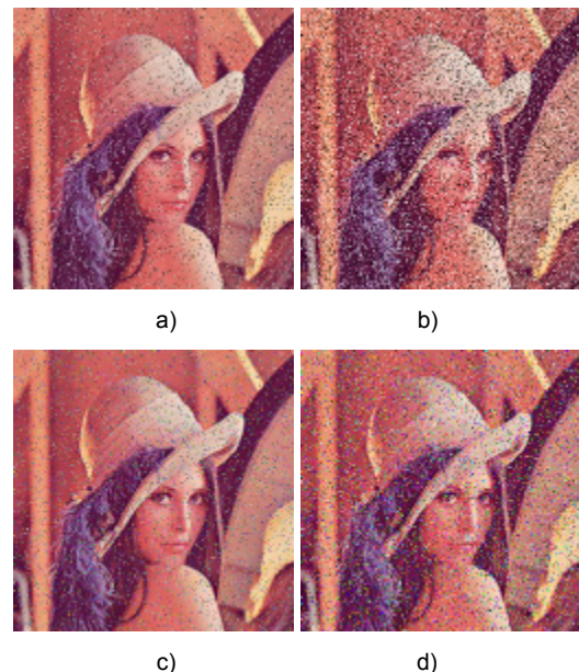
Fig. 2 The distorted images of the Lena: a) correlated impulsive, b) correlated salt and pepper, c) non-correlated impulsive, d) non-correlated salt and pepper
