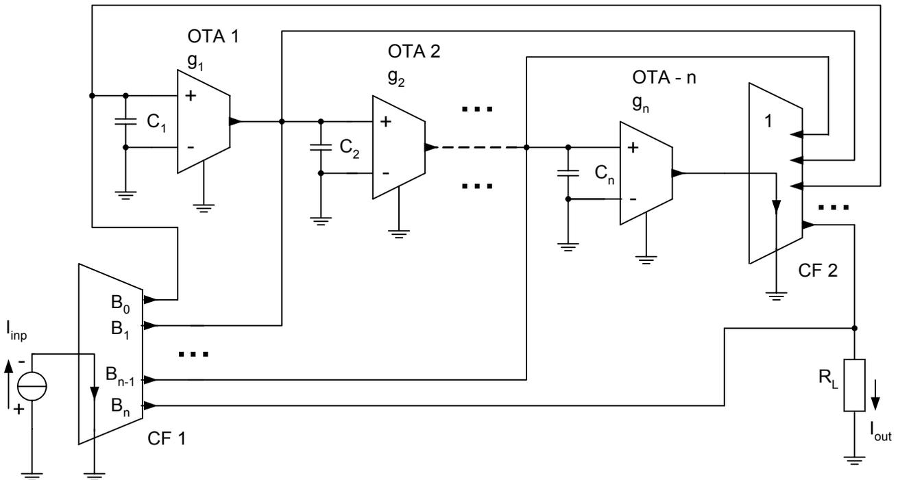
Fig. 4. Circuit diagram of the current mode  $n^{\text{th}}$ -order universal filter based on the inverse follow the leader feedback multi-loop structure with input distribution (IFLF-ID, Fig. 1d)
