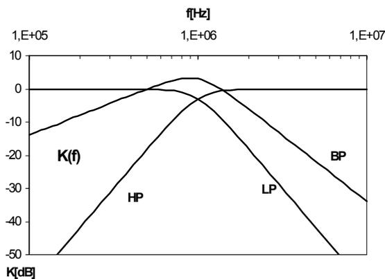
Fig. 2. Magnitude responses of the given 3<sup>rd</sup>-order filter.
