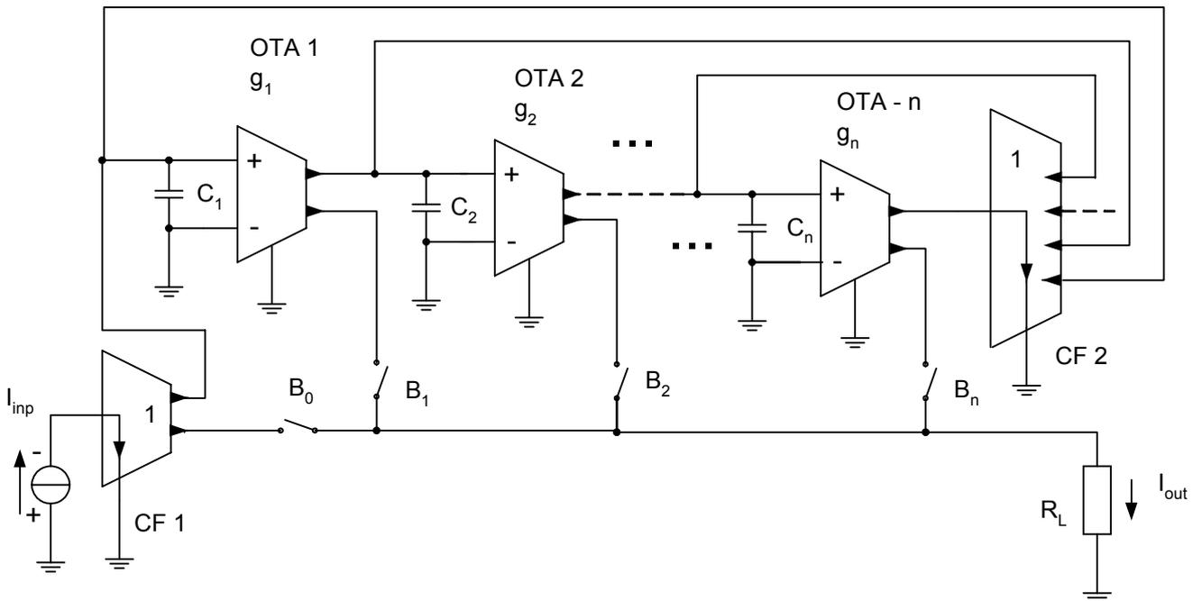
Fig. 6. Circuit diagram of the current mode  $n^{th}$ -order universal filter based on the inverse follow the leader feedback multi-loop structure with output summation (IFLF-OS, Fig. 1b).
