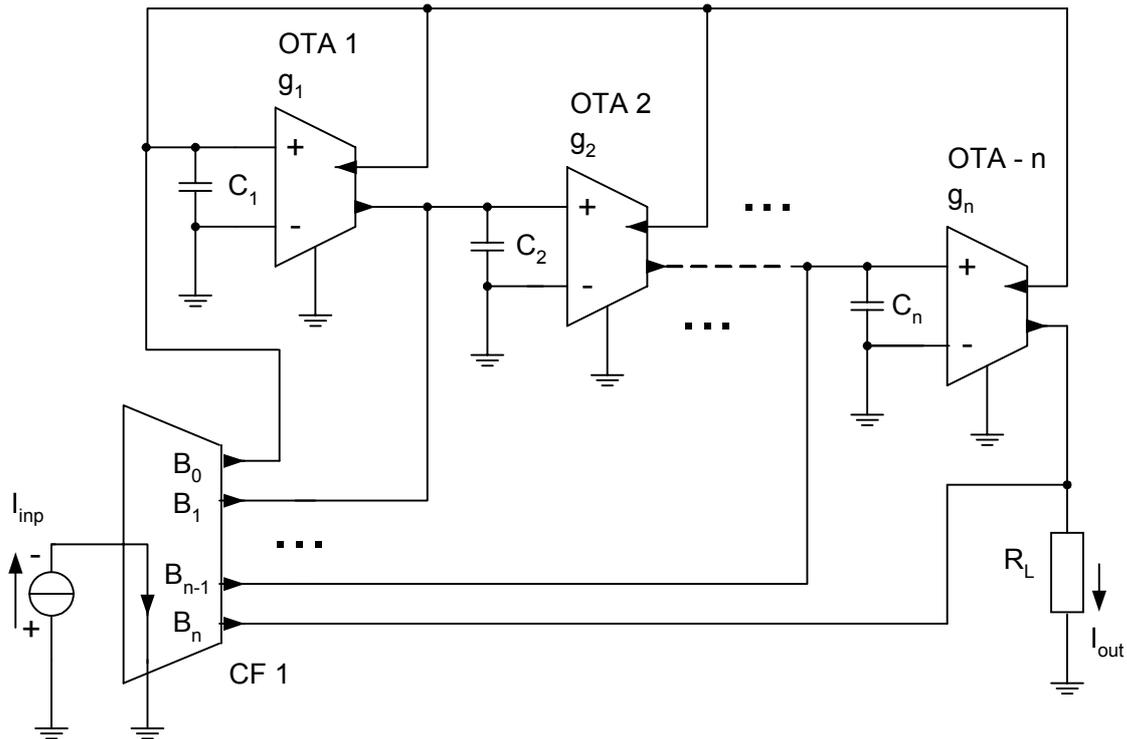
Fig. 3. Circuit diagram of the current mode  $n^{\text{th}}$ -order universal filter based on the follow the leader feedback multi-loop structure with input distribution (FLF-ID), corresponding with the signal flow graph given in Fig.2 (Fig. 1c).
