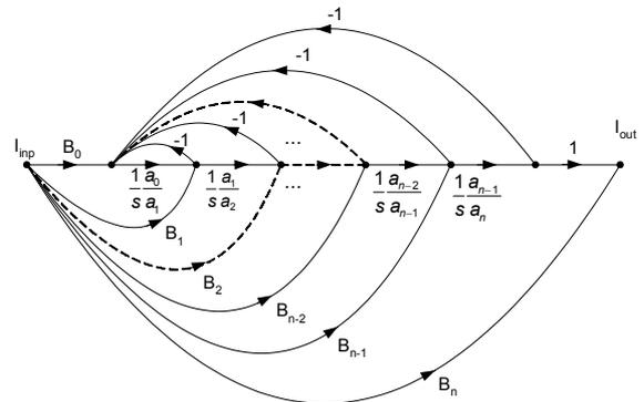
**Fig. 2.** Modification of the signal flow graph (Fig. 1c) of the multi-loop structure FLF-ID (Follow the leader feedback, with input distribution).
