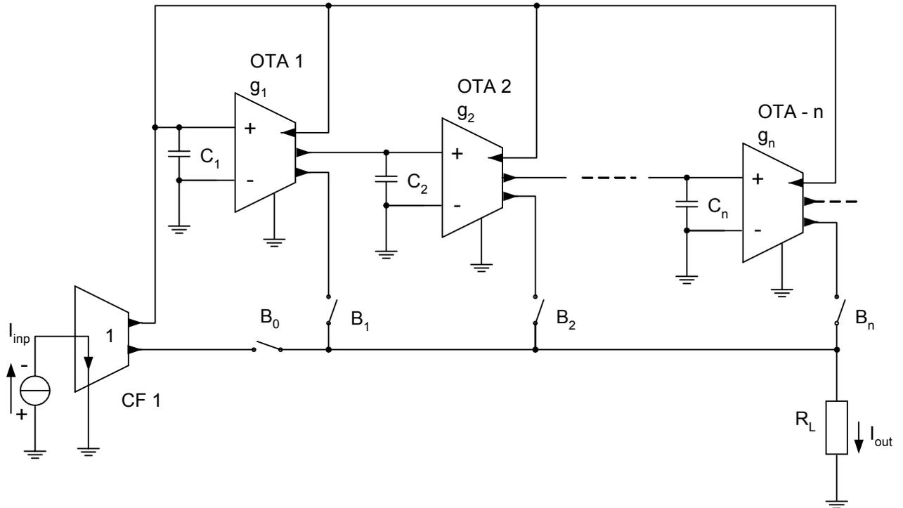
Fig. 5. Circuit diagram of the current mode  $n^{th}$ -order universal filter based on the follow the leader feedback multi-loop structure with output summation (FLF-OS, Fig. 1a).
