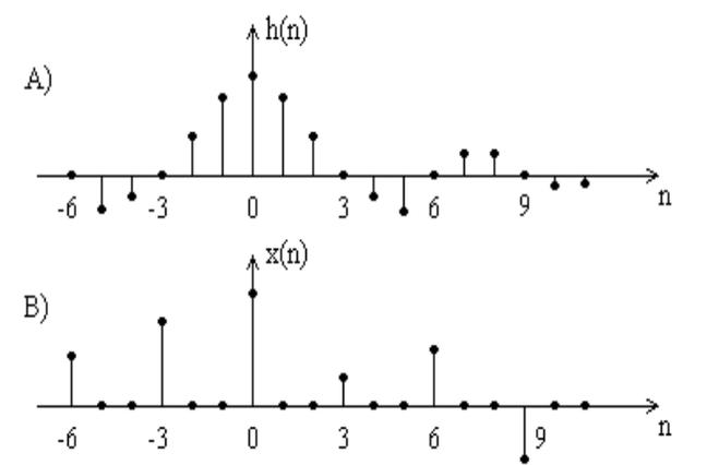
Fig. 3. Impulse response of the Nyquist- $M$  filter (A) and example of the input sequence (B).
