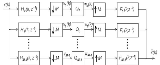
**Fig. 1.** Multirate subband coder for WSCS signals with maximally decimated filter bank.
