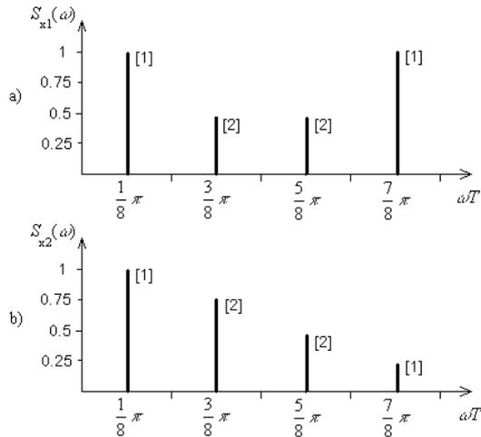
Fig. 7. Discrete spectra of input test waveforms, (A) defined by formula (3.1) and (B) formula (3.2).
