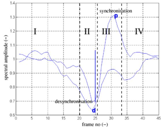
Fig. 1. Person 4, electrode 25, 10-23 Hz band. Vertical thin line denotes the time instant of the movement; D is the distal, P proximal movement. Total power in the band is depicted here. Around the time instant of movement strong desynchronization takes place, immediately after the movement is obvious synchronization (see [8])
