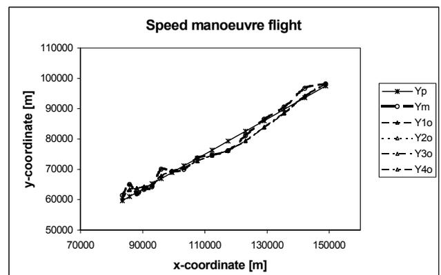
Fig. 4. Results of modeling the track of moving air object for section of track with direct unsteady movement.
