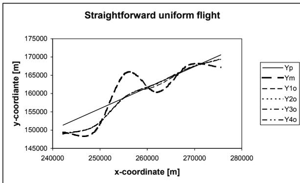
Fig. 1. Results of model tracking aircraft flight for section of rectilinear equal flying of aircraft (Direct, steady flight of aircraft).
