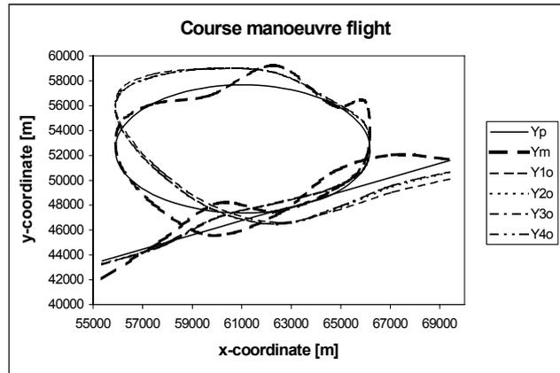
Fig. 2. Results of modeling track of flying aircraft for the section of tracking flight of the aircraft with left loop at 360°.
