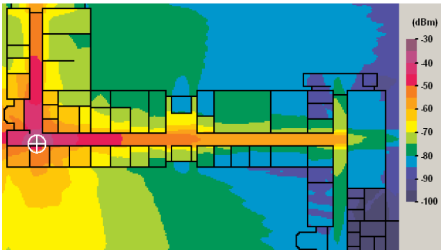
Fig. 7. Coverage prediction by a deterministic model [12]
