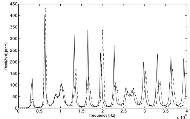
Fig. 11. The real part of the automotive FM antenna input impedance measured in the time (dashed line) and the frequency (solid line) domain.
