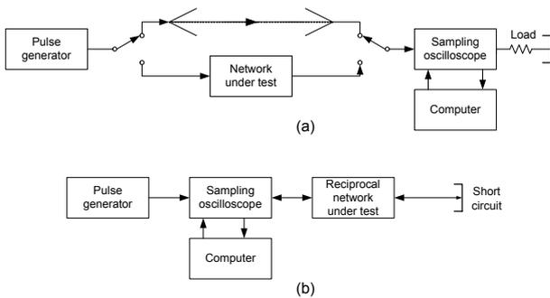
Fig. 2. Basic measurement configurations for transmission measurements.
