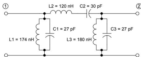
Fig. 4. The circuit diagram of the band pass filter measured in the time domain.
