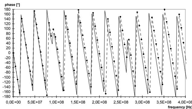
Fig. 10. The measured reflection phase of the automotive FM antenna in the time domain (dashed line with dots) and in the frequency domain (solid line).
