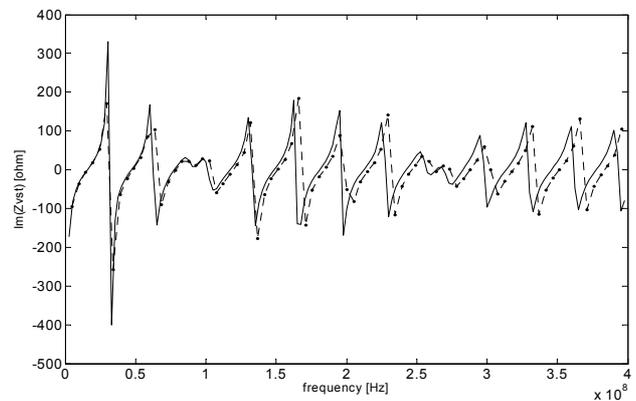
Fig. 12. The imaginary part of the automotive FM antenna input impedance measured in the time (dashed line) and the frequency (solid line) domains.
