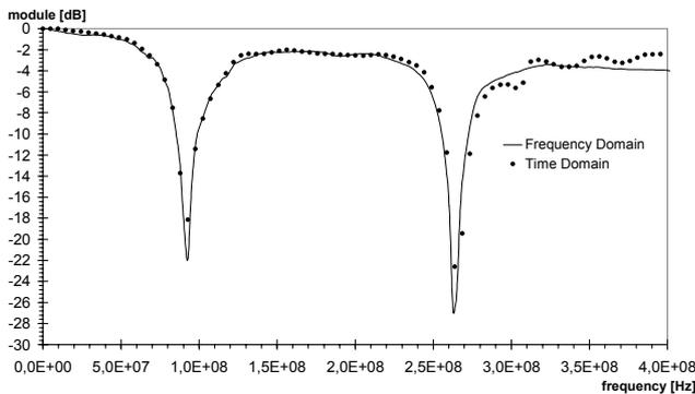
Fig. 9. The measured reflection amplitude of the automotive FM antenna.
