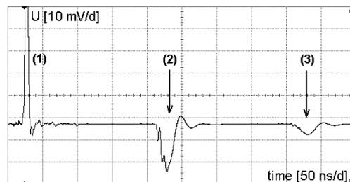
Fig. 8. Time separated waveforms (1) the generated pulse, (2) the reflected pulse, (3) multiple reflections.
