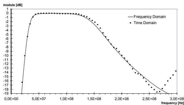
Fig. 5. The measured transmission amplitude of the band pass filter.
