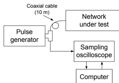
Fig. 7. The reflection measurement in the time domain arrangement.
