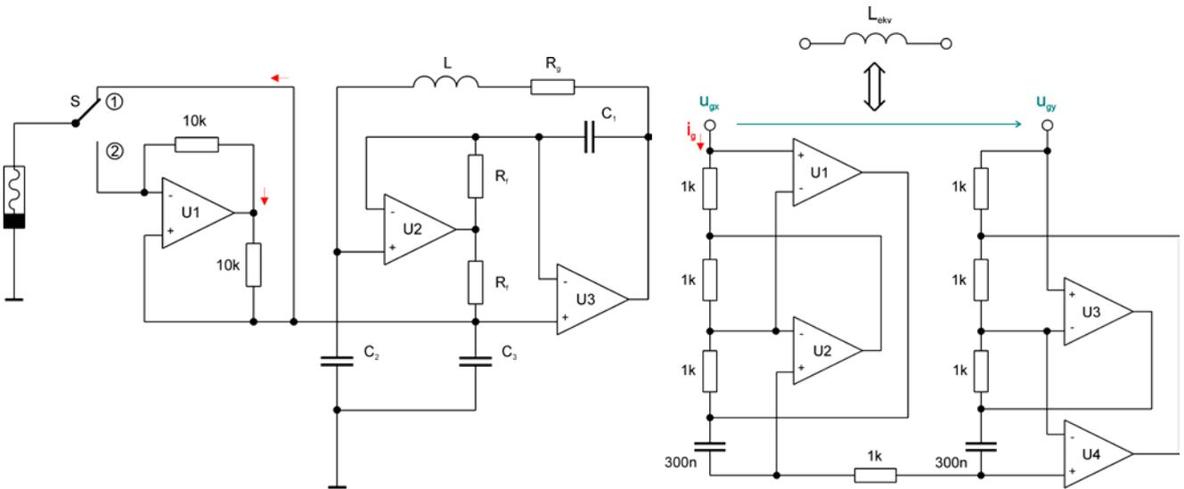
Fig. 10. Circuit implementation of universal chaos generator.
