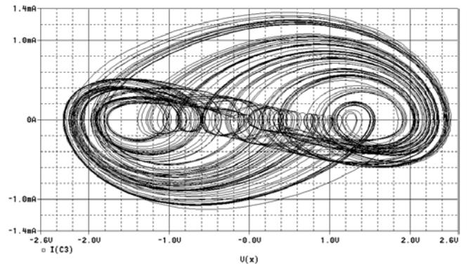
Fig. 6. I(C3)-V(C3) plane projection of the double scroll attractor.
