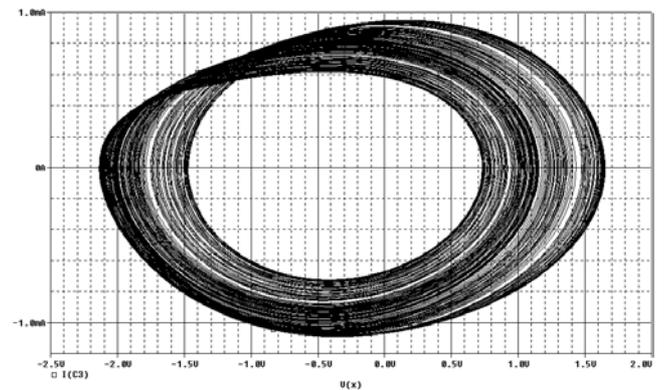
Fig. 7. I(C3)-V(C3) plane projection of the torus.
