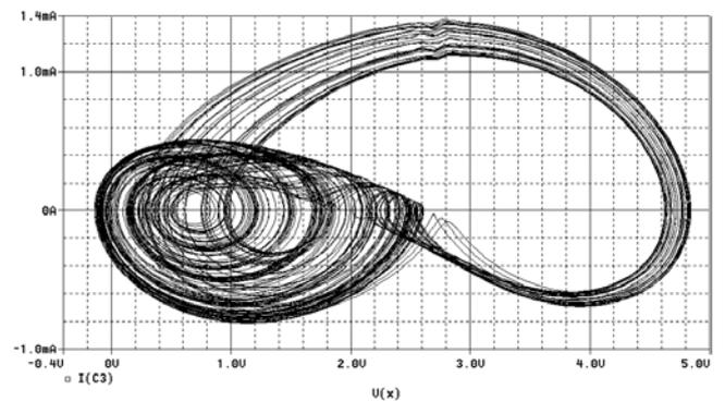
Fig. 8. I(C3)-V(C3) plane projection of the transition event.
