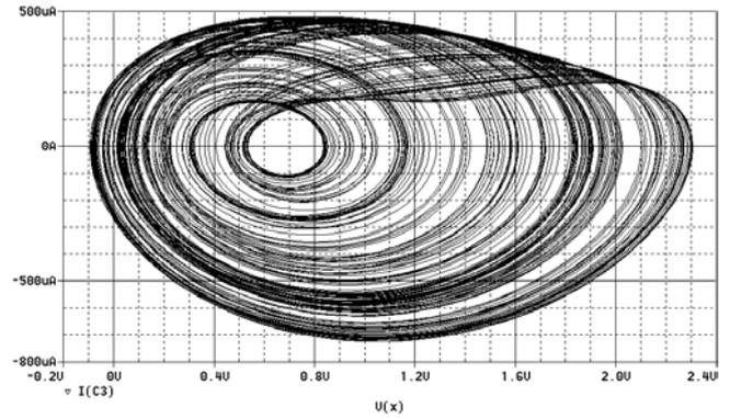
Fig. 5. I(C3)-V(C3) plane projection of the single scroll attractor.
