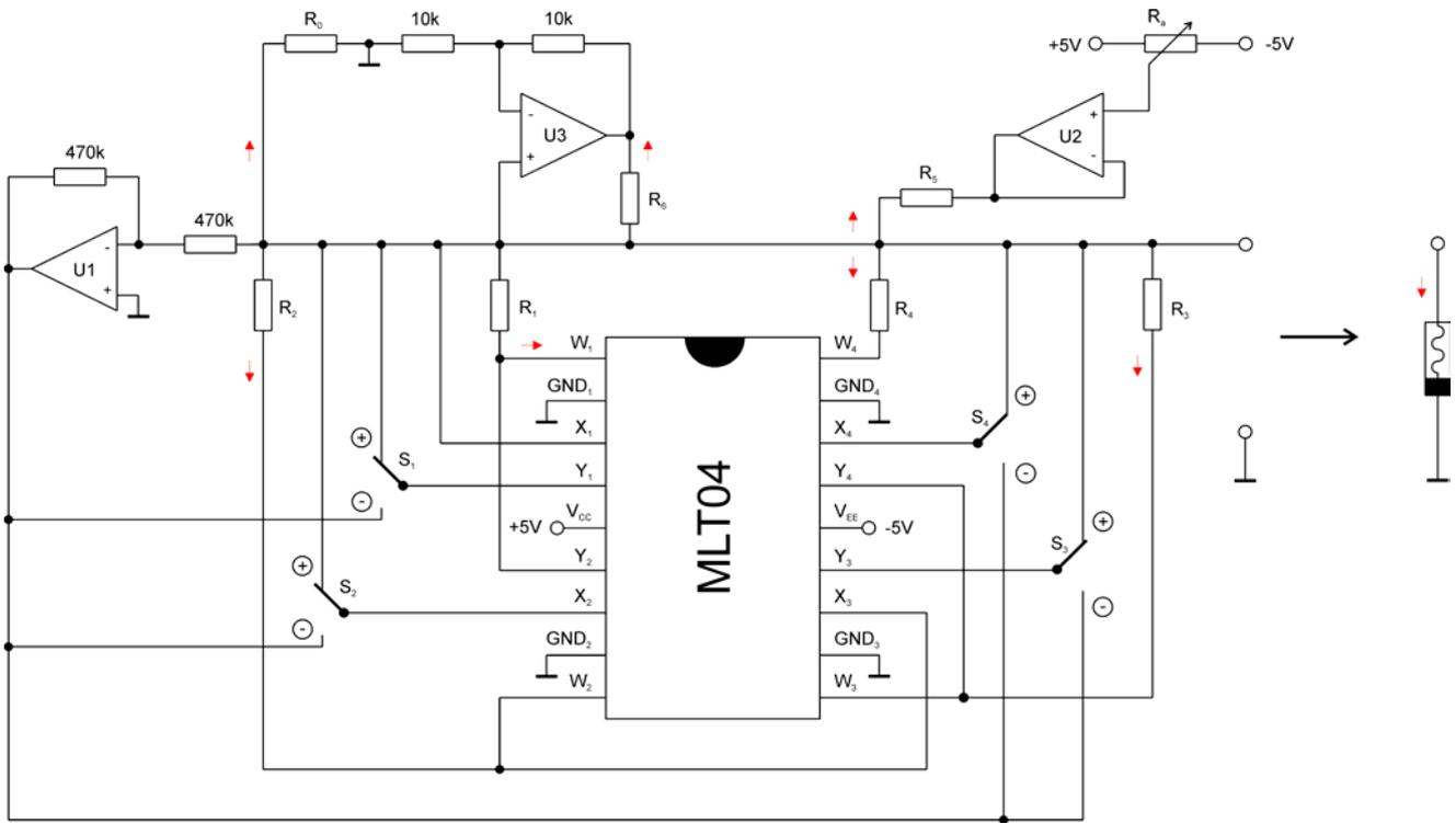
Fig. 9. Circuit implementation of polynomial resistive element (with current arrow convention).
