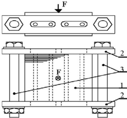
Fig. 1. The sketch of elastomagnetic sensor EMS-200kN, 1 – sheets, 2 – flanges, 3 – screws.
