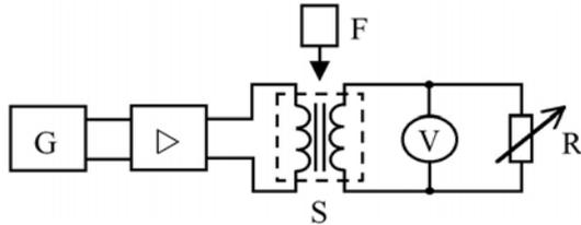
Fig. 4. The measuring apparatus.
