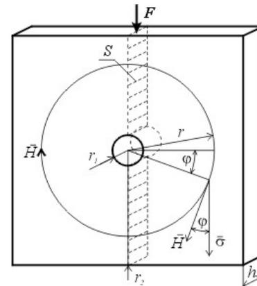
Fig. 2. The detail of a sheet element of an elastomagnetic sensor.
