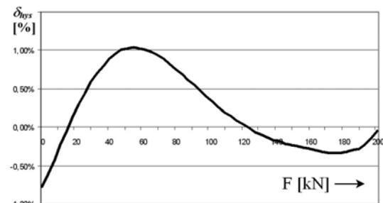
Fig. 7. The characteristic of hysteresis error.
