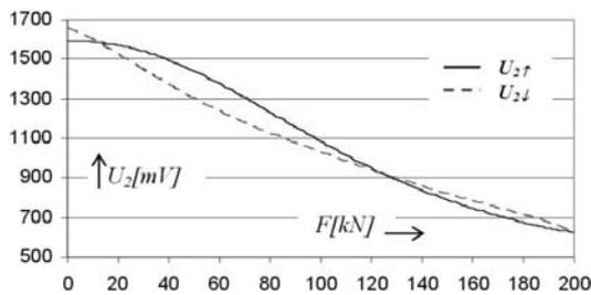
Fig. 5. The measured dependence of the output voltage  $U_{2\uparrow}=f(F)$  and  $U_{2\downarrow}=f(F)$ .
