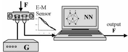
Fig. 8. The proposed solution of error reduction of EMS-200kN.
