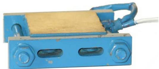
Fig. 3. Elastomagnetic sensor EMS-200kN.
