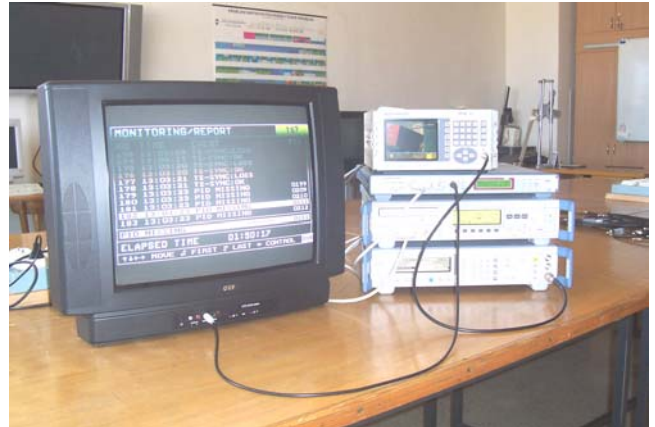
Fig. 3. The workplace for measurement of digital signals of the DVB-T standard.
