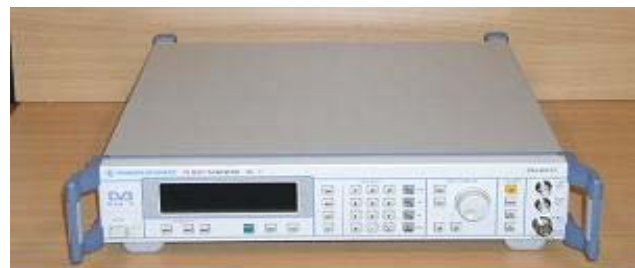
Fig. 1. Measuring test transmitter SFL-T (Rohde-Schwarz).
