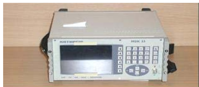
Fig. 2. Measuring receiver and analyzer MSK 33 (Kathrein).
