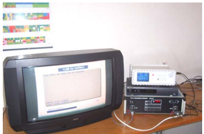
Fig. 4. The workplace for receiving of and measurement of digital signals of the DVB-S standard.
