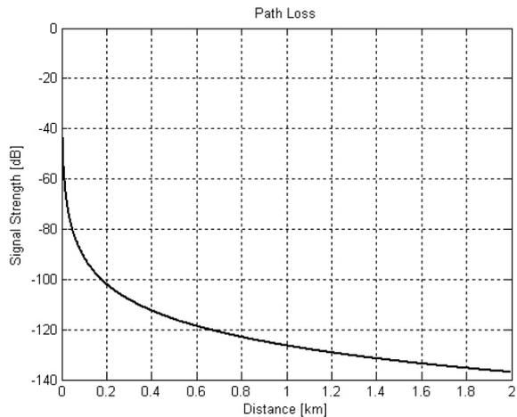
Fig. 5. Path Loss in urban environment according to (1).
