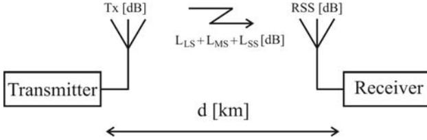
Fig. 3. RSS measurement model.
