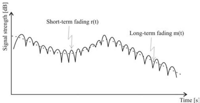
Fig. 1. A mobile radio signal fading representation.
