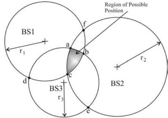
Fig. 4. The Region of Possible Positions formed by the Intersection of Circles.
