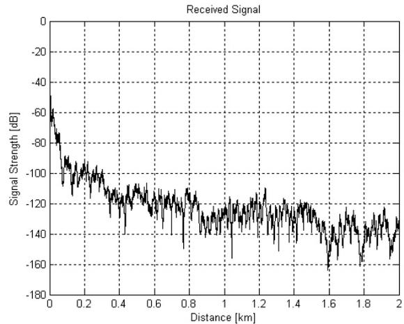
Fig. 4. Signal strength of mobile radio signal in urban environment.
