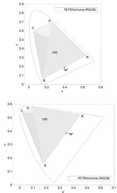
Fig. 5. One possibility of division of RGB color gamut of Tetra-chroma<sup>3</sup> Display Unit into sphere of activity of individual sub-gamuts shown in CIE xy (top) and CIE u'v' (bottom) chromaticity diagram.
