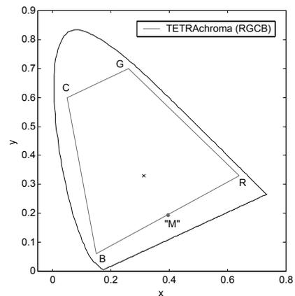
Fig. 3. Primaries of Tetra-chroma<sup>3</sup> Display Unit in the CIE xy chromaticity diagram.
