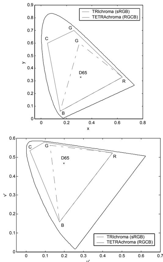
Fig. 1. Conventional sRGB and proposed RGC<sub>B</sub> color gamut in CIE  $xy$  (top) and CIE  $u'v'$  (bottom) chromaticity diagram.
