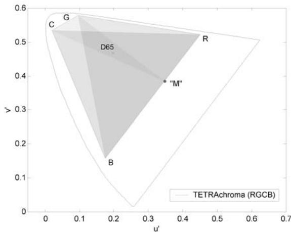
**Fig. 4.** Three sub-regions of RGCB tetragon of Tetra-chroma<sup>3</sup> Display Unit shown in CIE xy (top) and CIE u'v' (bottom) chromaticity diagrams.
