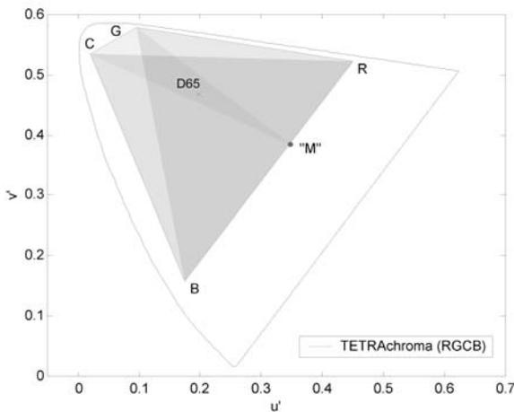
**Fig. 4.** Three sub-regions of RGCB tetragon of Tetra-chroma<sup>3</sup> Display Unit shown in CIE xy (top) and CIE u'v' (bottom) chromaticity diagrams.
