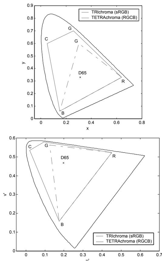
Fig. 1. Conventional sRGB and proposed RGCB color gamut in CIE  $xy$  (top) and CIE  $u'v'$  (bottom) chromaticity diagram.
