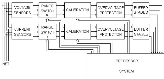
Fig. 1. Block diagram of the proposed digital electricity meter.
