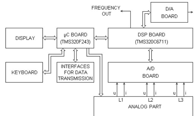
Fig. 3. Block diagram of the digital part of the proposed electricity meter.
