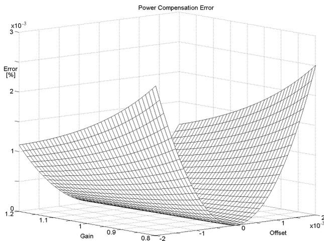
Fig. 5. Power correction error of the simplified calculation procedure.
