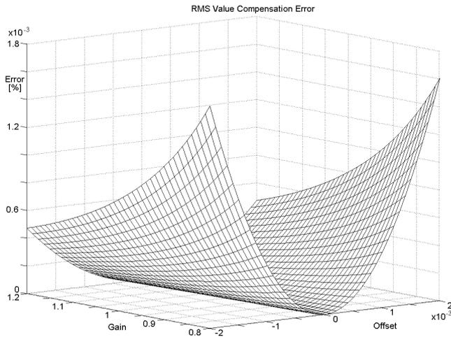
Fig. 4. RMS value correction error of the simplified calculation procedure.
