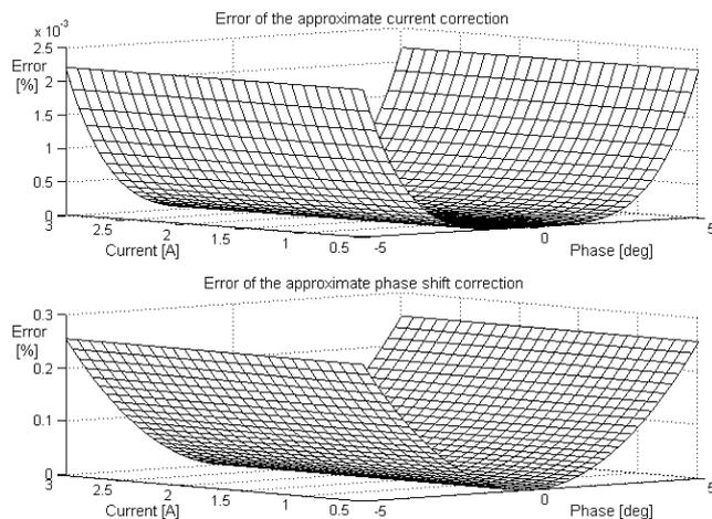
Fig. 6. Errors of the approximate current and phase shift corrections.
