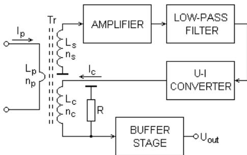
Fig. 2. Block diagram of the compensated current transformer.
