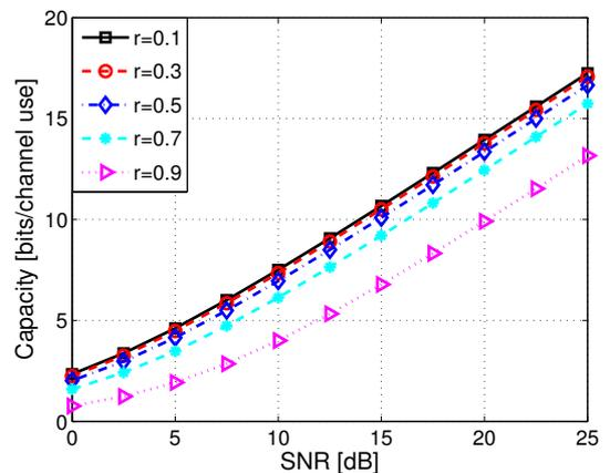
**Fig. 10.** Capacity—Eigenmode sub-space total channel inversion under correlated fading,  $N_R = N_T = 3$ .
