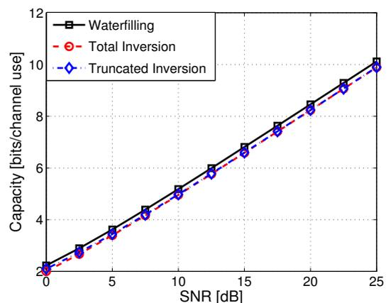
**Fig. 11.** Capacity—Alamouti scheme with optimal waterfilling allocation versus sub-optimal inversion,  $N_R = N_T = 2$ .
