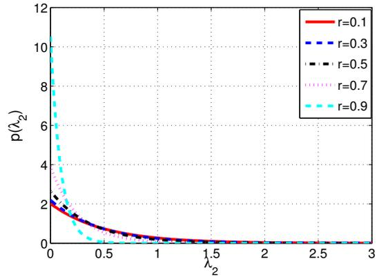
Fig. 5. The weakest eigenmode marginal density function,  $p(\lambda_2)$  under correlated fading,  $N_T = N_R = 2$ .
