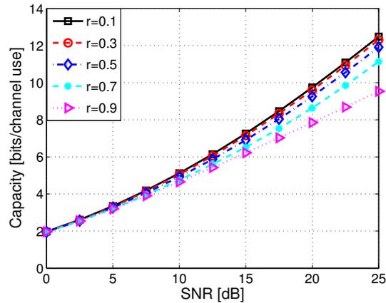
Fig. 7. Capacity—Eigenmode full-space truncated channel inversion under correlated fading,  $N_R = N_T = 2$ .
