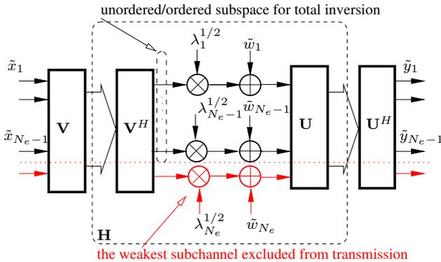
Fig. 2. SVD, reduced space of eigenmodes.
