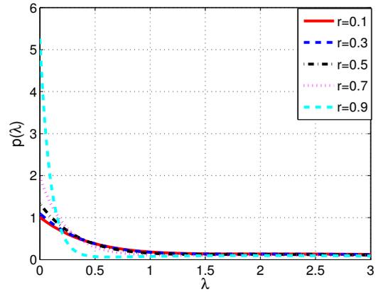
Fig. 6. The shared eigenmode marginal density function (un-ordered case),  $p(\lambda)$  under correlated fading,  $N_T = N_R = 2$ .
