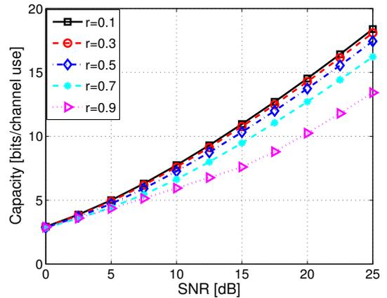
**Fig. 9.** Capacity—Eigenmode full-space truncated channel inversion under correlated fading,  $N_R = N_T = 3$ .
