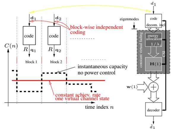
Fig. 1. System model and coding approach.
