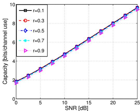
**Fig. 8.** Capacity—Eigenmode sub-space total channel inversion under correlated fading,  $N_R = N_T = 2$ .
