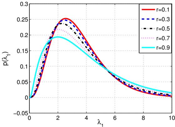
Fig. 4. The strongest eigenmode marginal density function,  $p(\lambda_1)$  under correlated fading,  $N_T = N_R = 2$ .
