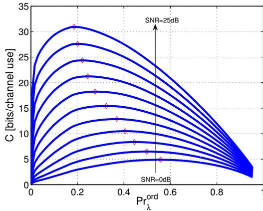
**Fig. 12.** Transmission outage probability versus capacity trade-off,  $N_T = N_R = 5$ ,  $\text{SNR} = \{0; 2.5, \dots, 25\}$  dB.
