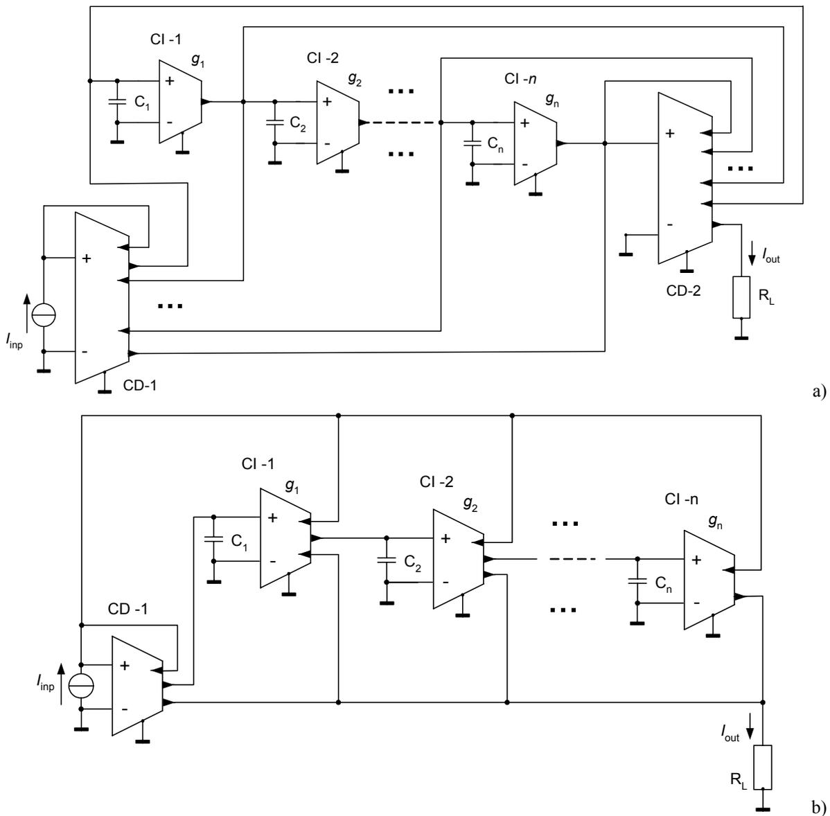
Fig. 5. Circuit diagram of the current mode  $n^{th}$ -order all-pass filter with the OTAs
