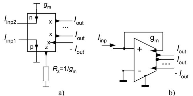
**Fig. 4.** Multi-output current distributors: a) using CDTA-CDIMO, b) using OTA-SIMO.
