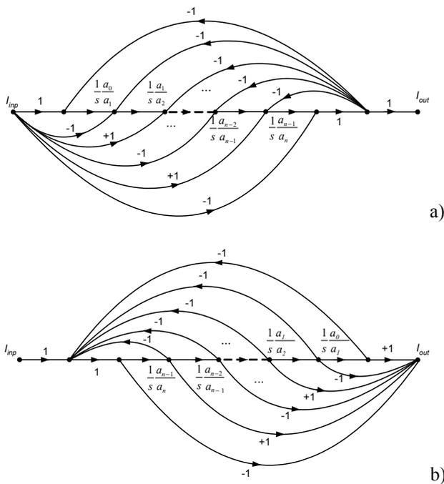
**Fig. 2.** Modified signal flow graphs of the multi-loop structures convenient for  $n^{\text{th}}$ -order all-pass filter in the current mode:
