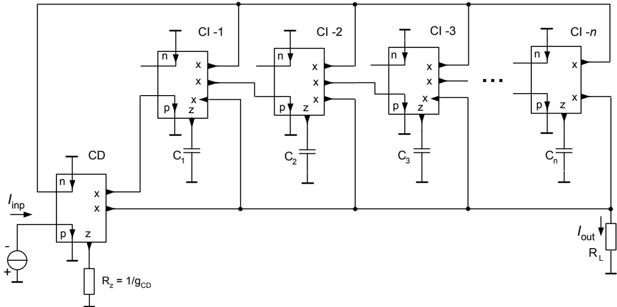
Fig. 6. Circuit diagram of the current mode  $n^{th}$ -order all-pass filter with the CDTAs based on the second canonical structure (FLF-OS), corresponding to the SFG given in Fig.2b.
