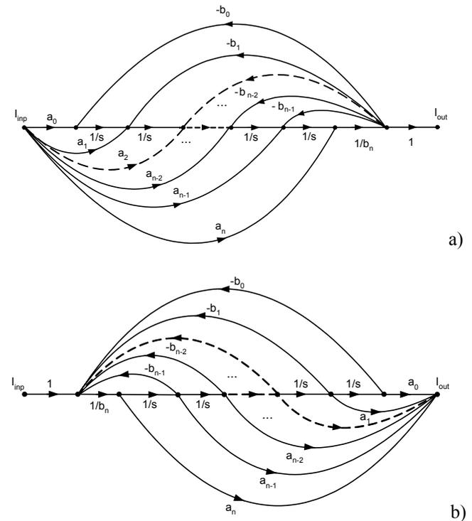
**Fig. 1.** Basic signal flow graphs of the multi-loop structures in the current mode.
