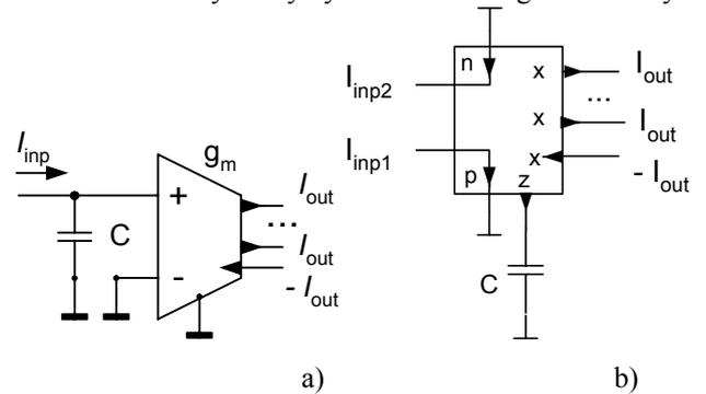
**Fig. 3.** Multi-output current integrators.
