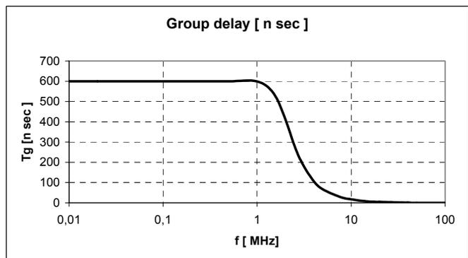
Fig. 9. Group delay response of the designed 4<sup>th</sup>-order filter.
