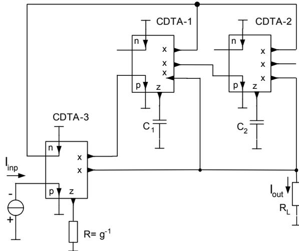
Fig. 8. Second-order all-pass filters with the CDTAs.
