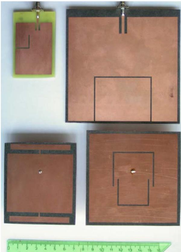
**Fig. 1.** The photograph of compared antennas: the L-slot antenna (top left), the double-extended antenna (bottom left), the U-slot antenna (top right), and the double-U antenna (bottom right).
