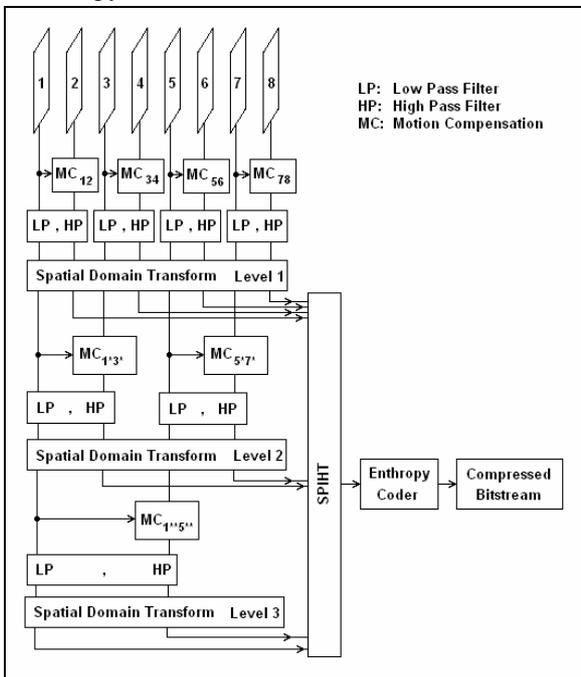
Fig.3. Motion Compensated 3D Wavelet Encoder
