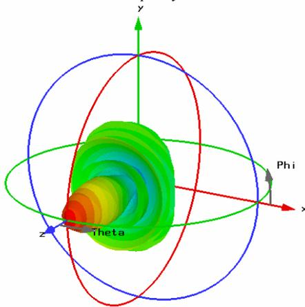
Fig. 10. Directivity pattern of the antenna completed by the dielectric lens at the frequency 100 GHz.
