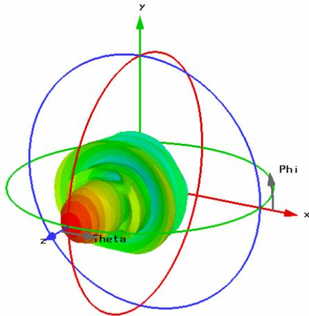
Fig. 9. Directivity pattern of the antenna completed by the dielectric lens at the frequency 80 GHz.
