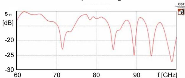
**Fig. 16.** Return loss of the horn antenna completed by the metallic lamellas.
