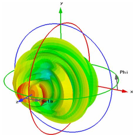
Fig. 13. Directivity pattern of the optimized antenna with metallic lamellas at the frequency 60 GHz.
