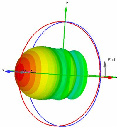
Fig. 3. Directivity pattern of the original horn antenna at the frequency 60 GHz.
