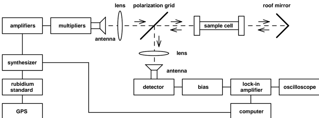
Fig. 1. Block diagram of a molecular spectroscope.
