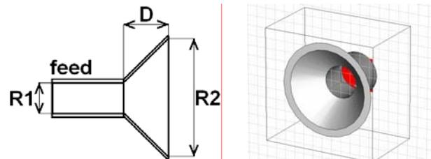
Fig. 2. Basic geometry of the original horn antenna.
