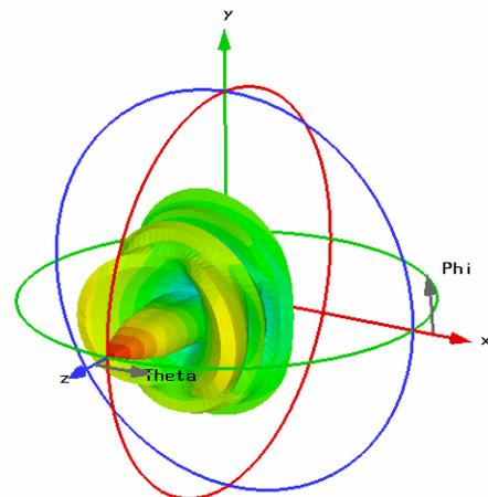
Fig. 14. Directivity pattern of the optimized antenna with metallic lamellas at the frequency 80 GHz.
