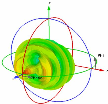
**Fig. 15.** Directivity pattern of the optimized antenna with metallic lamellas at the frequency 100 GHz.
