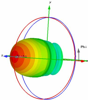
Fig. 4. Directivity pattern of the original horn antenna at the frequency 80 GHz.
