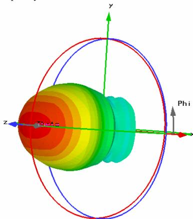
Fig. 5. Directivity pattern of the original horn antenna at the frequency 100 GHz.
