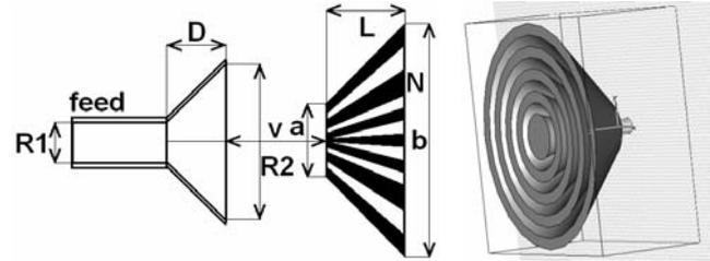
Fig. 12. Optimized horn antenna with metallic lamellas.
