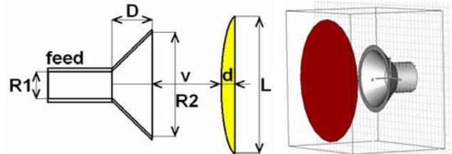
Fig. 7. Horn antenna with the dielectric lens
