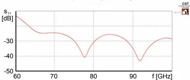
Fig. 11. Return loss of the horn antenna completed by the dielectric lens.
