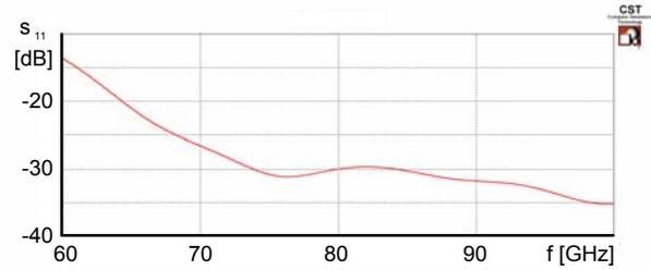
Fig. 6. Return loss of the original horn antenna.
