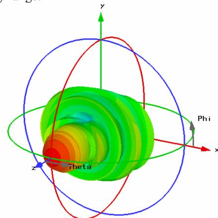
Fig. 8. Directivity pattern of the antenna completed by the dielectric lens at the frequency 60 GHz.
