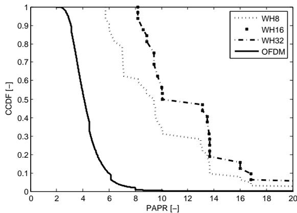
Fig. 3. CCDF of PAPR for no interleaving and spreading sequence (Walsh spreading sequences) length 8 (WH8), 16 (WH16) and 32 (WH32).
