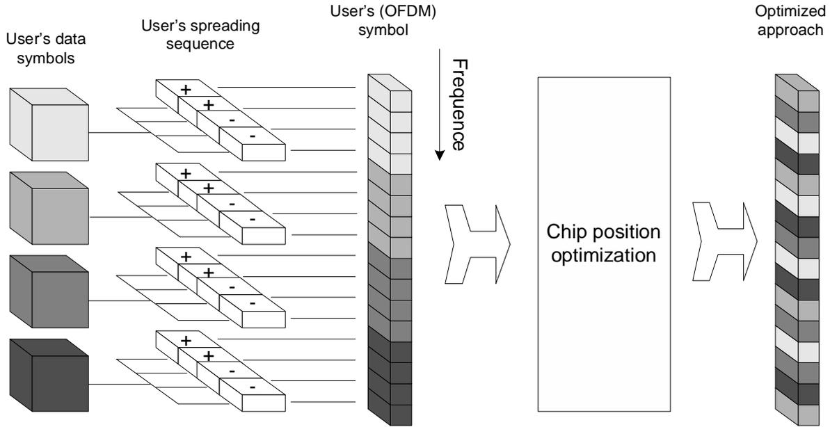
Fig. 1. M-modification of MC-CDMA and its optimization.
