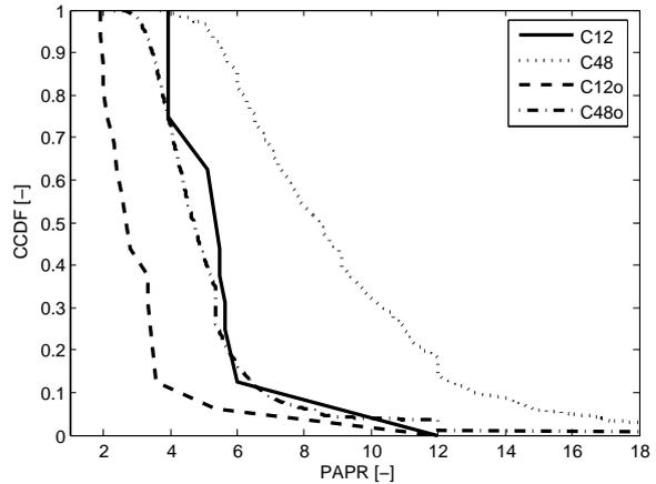
Fig. 2. CCDF of PAPR for different number of subcarriers - 12 subcarriers with (C12o) and without (C12) optimization, and 48 subcarriers with (C48o) and without (C48) optimization.
