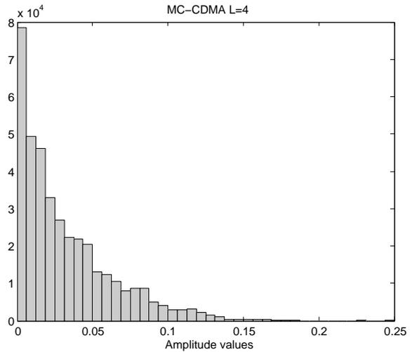
Fig. 5. Amplitude histogram for MC-CDMA, 32 subc. L=4, BPSK.
