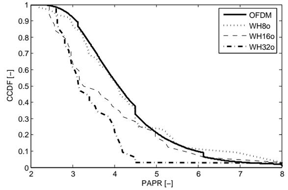
Fig. 4. CCDF of PAPR for optimized interleaving and spreading sequence (Walsh spreading sequences) length 8 (WH8o), 16 (WH16o) and 32 (WH32o).
