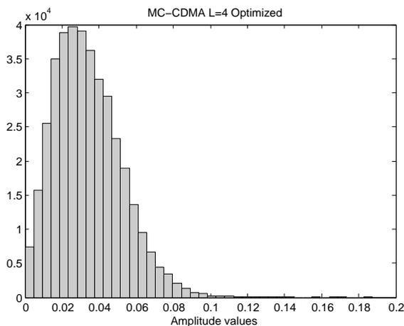
Fig. 6. Amplitude histogram for MC-CDMA, 32 subcarriers,  $L=4$ , BPSK with optimized interleaving.
