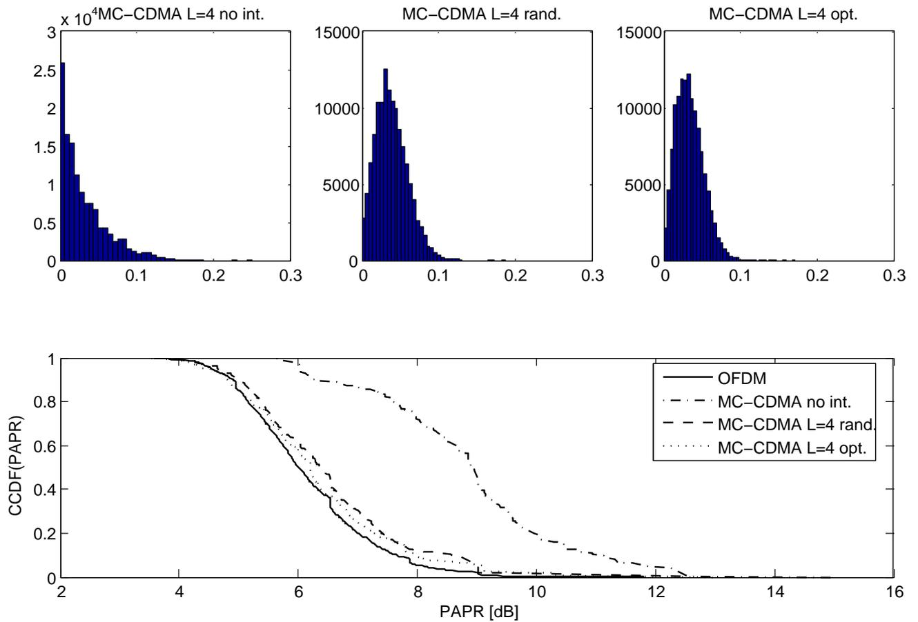
Fig. 7. Comparison of not interleaved, optimized and random interleaving for one user MC-CDMA with 32 subc., L=4 and BPSK modulation.
