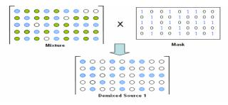
Fig. 1. Using binary time-frequency masking to recover the time-frequency representation of one source from the time- frequency representation of one mixture. At blue points source 1 is active, at green points source 2 is active, at white points no source is active. Note that the green points are completely masked.
