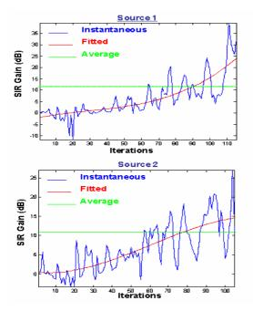
**Fig. 3.** The evolution of the SIR gains for two sources separated from two instantaneous mixtures. The overall average SIR gains are around 10 dB which is less due the convergence process in the first iterations of the algorithms. The average convergence time from different tests is 1.4 sec.
