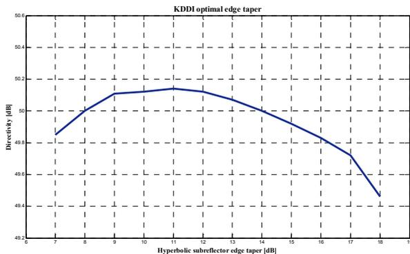
Fig. 4. Subreflector edge taper characteristics.
