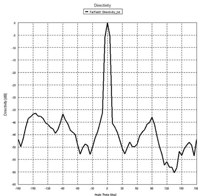
Fig. 10. 2 D Normalized Radiation Pattern 432MHz,  $\phi = 90^\circ$ .
