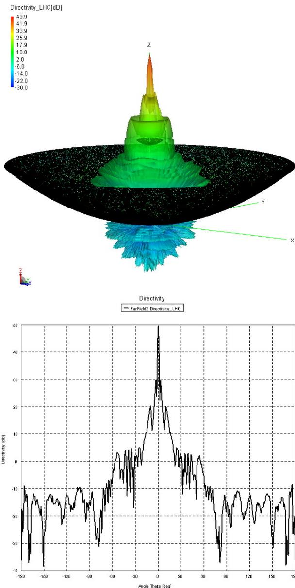
Fig. 6. Copolarization Radiation Pattern (3D) - above and 2D - below, at plane  $\phi = 90^\circ$
