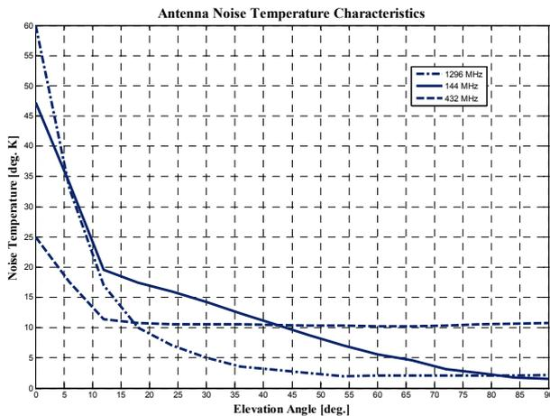
Fig. 12. The KDDI antenna calculated noise temperature characteristics.
