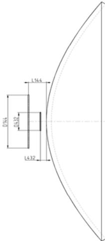
Fig. 7. 2m and 70cm loops geometry.
