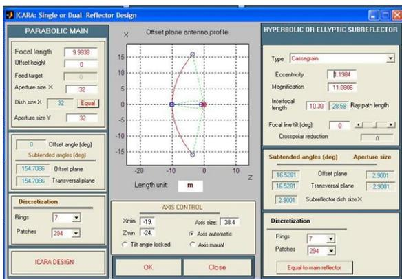
Fig. 2. Cassegrain antenna system in ICARA software.
