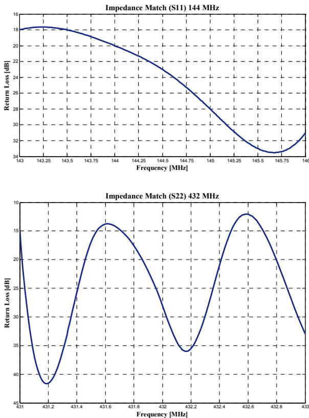
Fig. 8. Measured return loss of the loops, 2m (above), 70cm (below).
