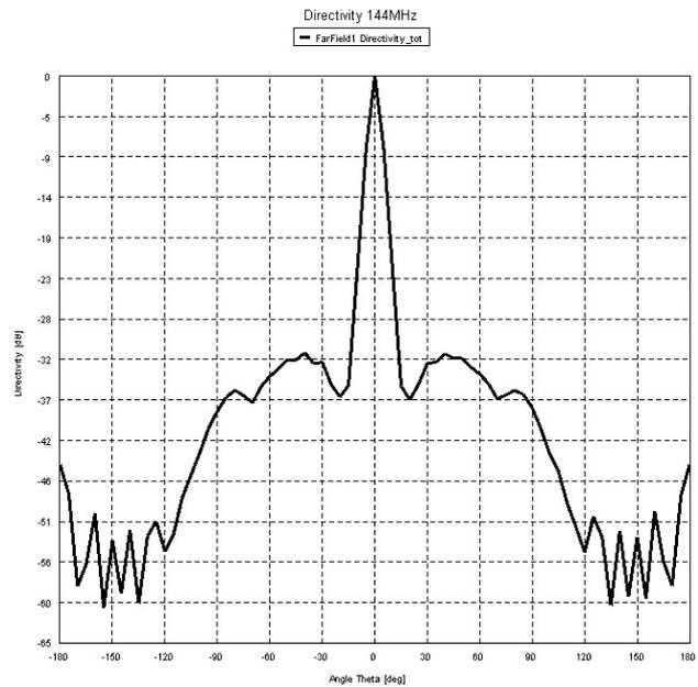
Fig. 9. 2 D Normalized Radiation Pattern 144 MHz,  $\phi = 90^\circ$ .
