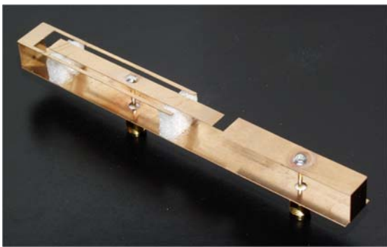
Fig. 3. Double PIFA for GSM/DCS (feed point to the left) and UMTS bands.
