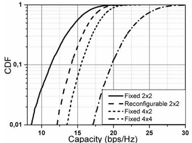
Fig. 4. CDF of the capacity for the fixed 2x2, 4x4, 4x2 and the reconfigurable 2x2 MIMO systems.
