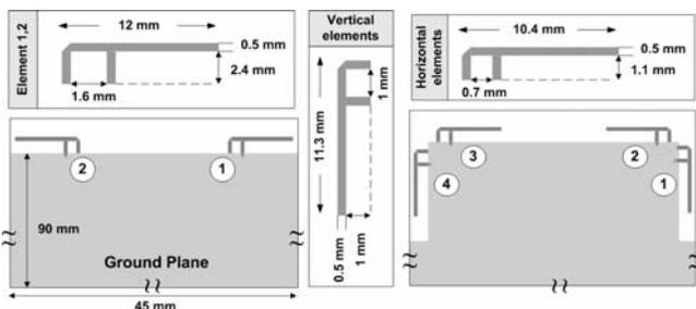
Fig. 1. The layout of the investigated compact common phase center MEA structures.
