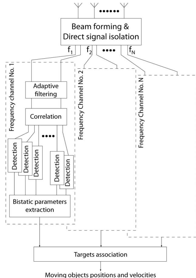
**Fig. 4.** A basic block diagram of the signal processing in CMS.
