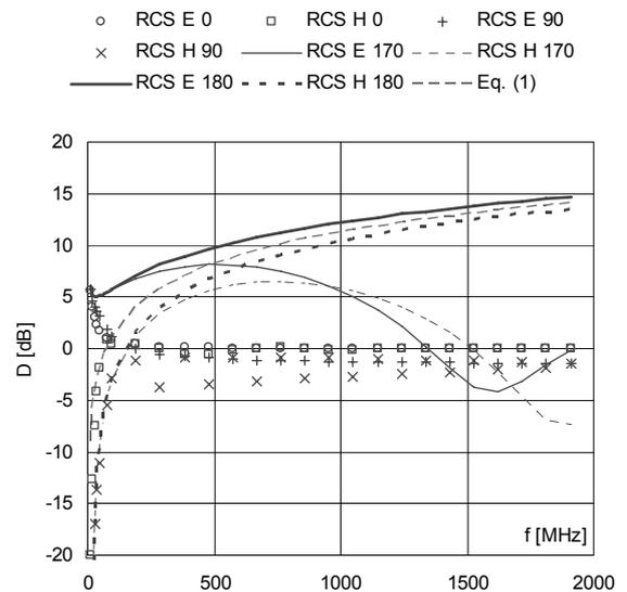
Fig. 2. Variations of  $D = 10 \log \sigma / ka^2$  for the perfectly conducting cylinder with radius of  $a = 0.5 \text{ m}$  (RCS E 90 indicates that incident electric field is parallel to the cylinder axis and bistatic angle is 90 degrees etc.).
