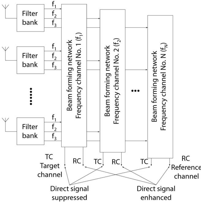
Fig. 5. Antenna subsystem - the direct and scattered signals separation.
