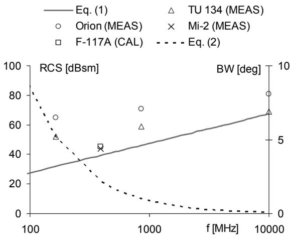
**Fig. 3.** Calculated forward scatter RCS  $\sigma_F$  and  $\theta_0$  for  $A = 20 \text{ m}^2$  and  $d = 20 \text{ m}$ . RCS  $\sigma_F$  calculation (F-117A [8]) and measurements (Mi-2 helicopter [8], TU 134 and Orion [5]).
