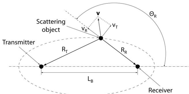
**Fig. 1.** Bistatic radar geometry:  $L_B$  is the length of the bistatic radar base,  $R_T$ ,  $R_R$  are the transmitter - object and object - receiver ranges,  $\Theta_R$  is the DOA angle of the received signal, scattered by the object.
