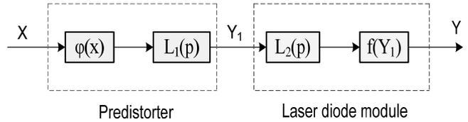
Fig. 2. Block diagram of PD-LD system described by Volterra series and Laplace transformations.
