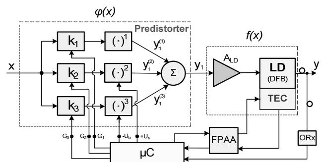
Fig.1. General block diagram for adaptive compensation of the laser diode' nonlinearity.
