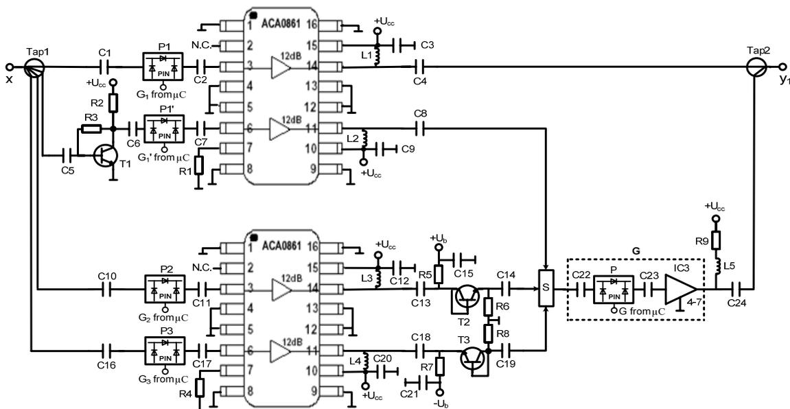
Fig.4. Predistorter electrical circuit diagram.
