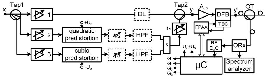
Fig.3. Block diagram for predistorter and the loop for adaptive compensation
