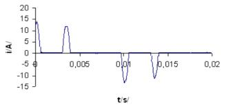
Fig. 3. Input converter current for 4 kW load.
