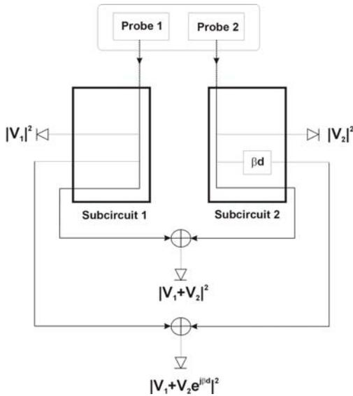
Fig. 1. Block diagram of hybrid probe for near-field phase retrieval.
