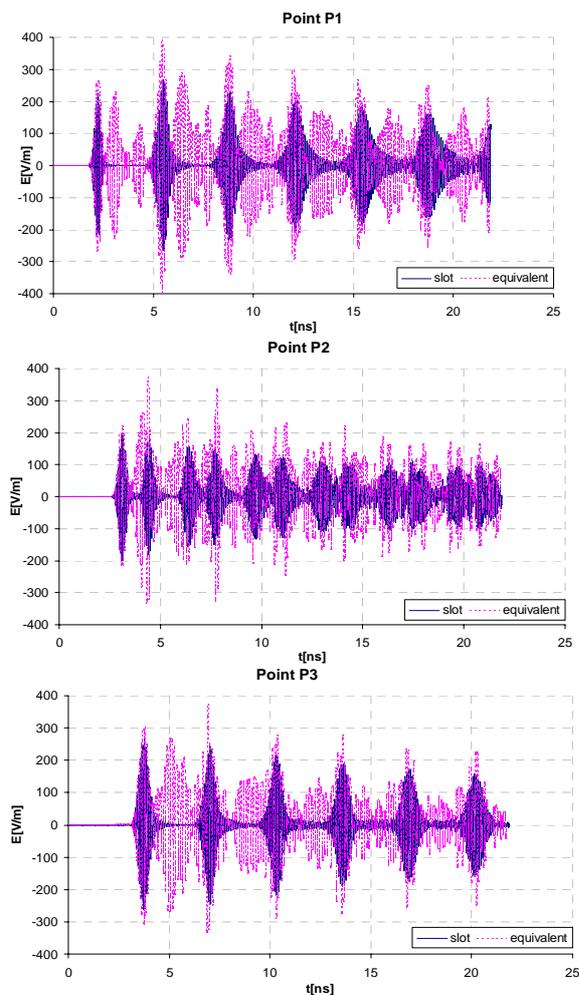
**Fig. 6.** Time response of field intensity in testing points for the angle of incidence  $60^\circ$ : the slot in composite (blue), the homogeneous equivalent (magenta).
