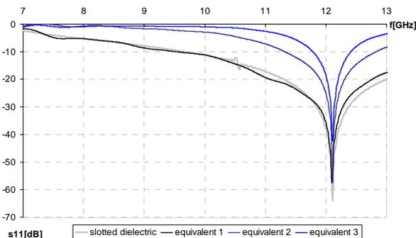
Fig. 2. Frequency response of the magnitude of the reflection coefficient for the slot in dielectric layer and for homogeneous equivalents specified in Tab. 1.
