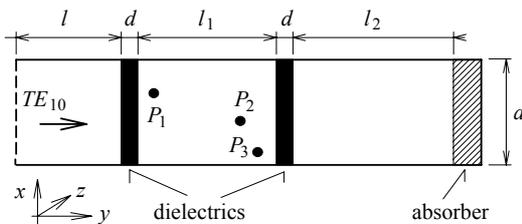
**Fig. 4.** The simplified airplane model. In  $P_1$  to  $P_3$ , virtual probes are assumed. Dimensions:  $l = l_1 = 370$  mm,  $l_2 = 180$  mm,  $d = 7$  mm,  $a = 22.86$  mm.
