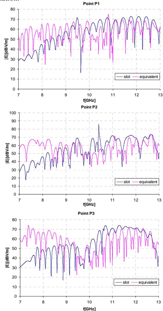
**Fig. 5.** Frequency response of field intensity in testing points for the angle of incidence  $60^\circ$ : the slot in composite (blue), the homogeneous equivalent (magenta).
