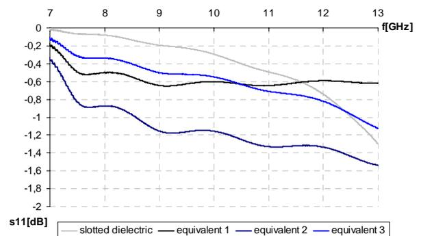
Fig. 3. Frequency response of the magnitude of the reflection coefficient for the slot in the composite material and for homogeneous equivalents specified in Tab. 2.
