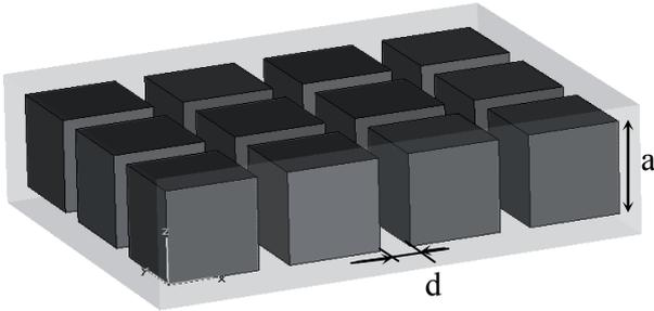
**Fig. 8.** The lattice of dielectric high permittivity cubes in the dielectric matrix of lower permittivity. The following parameters of cubes are used: size  $a = 3$  mm,  $\epsilon_r = 1000$ , dielectric cubes  $\tan \delta = 0.001$ , the distance between the cubes  $d = 1$  mm.
