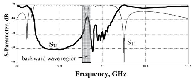
**Fig. 4.** Transmission  $S_{21}$  and reflection  $S_{11}$  coefficients for the structure depicted in Fig. 3. Gray area is the frequency range, where the resonant frequencies of two types of resonances coincide and backward wave is observed.
