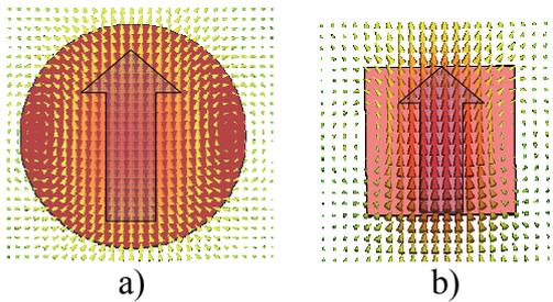
**Fig. 9.** Magnetic resonance in a) the dielectric spherical particle b) the dielectric cubic particle.
