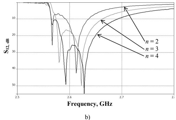
**Fig. 11.** a) Dielectric cubes structure with several number of cube layers. b) Transmission coefficient for different number  $n$  of layers,  $d = 3$  mm,  $h = 1.2$  mm.
