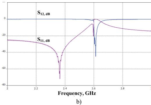
**Fig. 10.** a) 2 layer dielectric cube structure. b) Transmission and reflection coefficient for this structure  $d = 5$  mm,  $h = 5$  mm.
