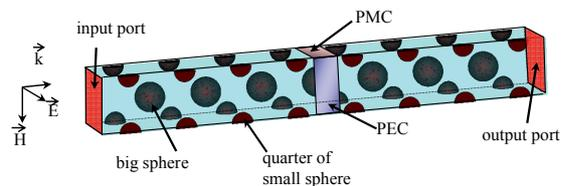
**Fig. 3.** 1-D structure of bi-spherical isotropic metamaterial. Radii of small and big spheres are 0.748 mm and 1.05 mm respectively. Boundary conditions are provided by perfect magnetic (PMC) and perfect electric (PEC) walls.
