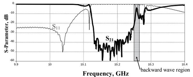
**Fig. 7.** Transmission  $S_{21}$  and reflection  $S_{11}$  coefficients for the modeled structure depicted in Fig. 5. Gray area is the frequency range where two types of resonances coincide and backward wave is observed.
