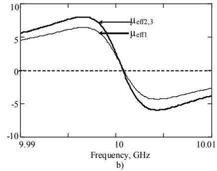
**Fig. 2.** Effective a) permittivity and b) permeability for face-centered Na-Cl structure (sub-index 1) the face-centered structure (sub-index 2) and body-centered structure (sub-index 3).
