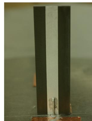
Fig. 13. Picture of a printed monopole antenna on magneto-dielectric material.
