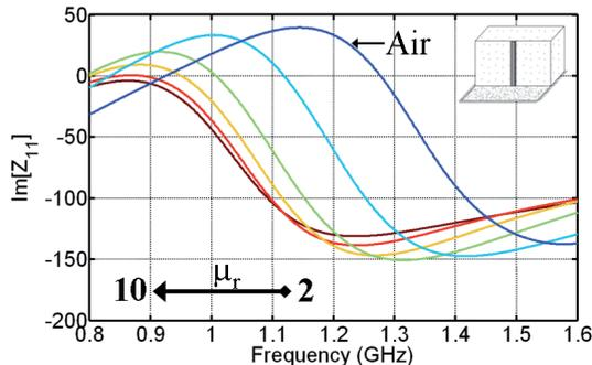
Fig. 6. Imaginary part of the input impedance with magnetic substrate.
