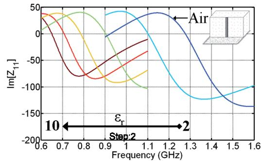
Fig. 4. Imaginary part of the input impedance with dielectric substrate.
