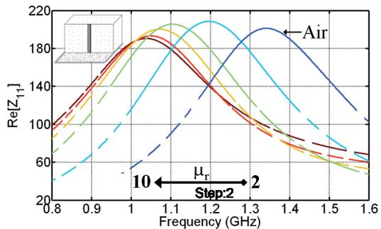
Fig. 5. Real part of the input impedance with magnetic substrate.
