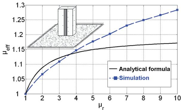
Fig. 9. Effective permeability vs relative permeability for an antenna printed on a magnetic substrate.
