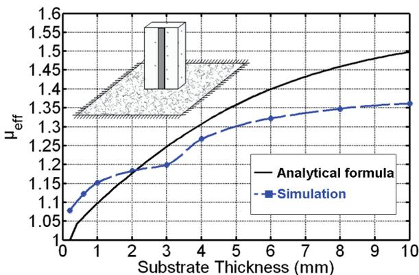
Fig. 11. Effective permeability vs substrate thickness for an antenna printed on a magnetic substrate.
