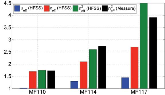
Fig. 16. Extraction of the effective permittivity  $\epsilon_{eff}$ , the effective permeability  $\mu_{eff}$  and the effective index  $n_{eff}^2$  versus different magnetodielectric materials.
