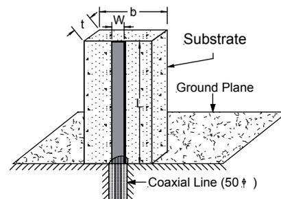
Fig. 1. Geometry of the printed monopole antenna.
