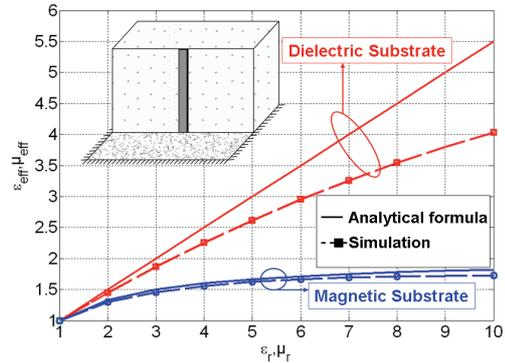
Fig. 7.  $\epsilon_{eff}$  and  $\mu_{eff}$  versus  $\epsilon_r$  and  $\mu_r$  respectively for a monopole antenna printed on a dielectric and a magnetic substrate.
