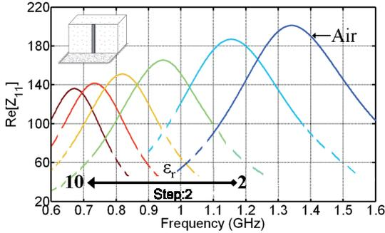
Fig. 3. Real part of the input impedance with dielectric substrate.
