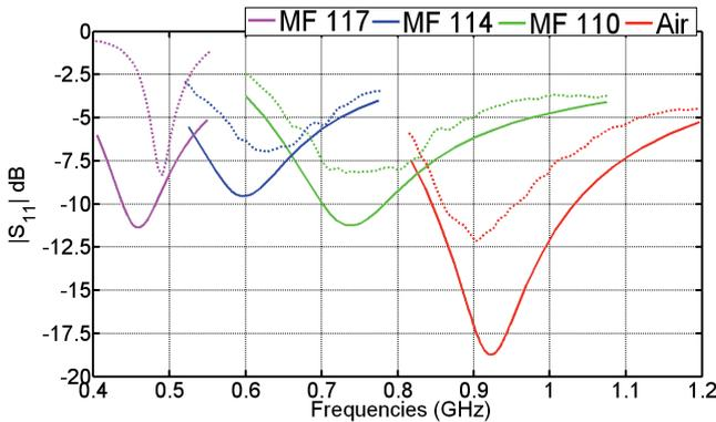
Fig. 15. Input reflection coefficient  $S_{11}$  of monopole antenna with the magnetodielectric materials : (dot) measured and (solid) simulation.
