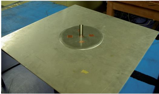
Fig. 14. Picture of a printed monopole antenna mounted over a large ground plane.
