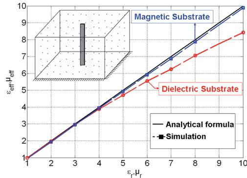
Fig. 8.  $\epsilon_{eff}$  and  $\mu_{eff}$  versus  $\epsilon_r$  and  $\mu_r$  respectively for a monopole antenna inside both homogeneous dielectric and magnetic substrate.
