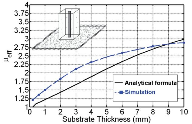
Fig. 12. Effective permeability vs substrate thickness for an antenna within a homogeneous magnetic substrate.
