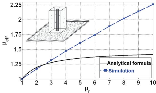
Fig. 10. Effective permeability vs relative permeability for an antenna within a homogeneous magnetic substrate.
