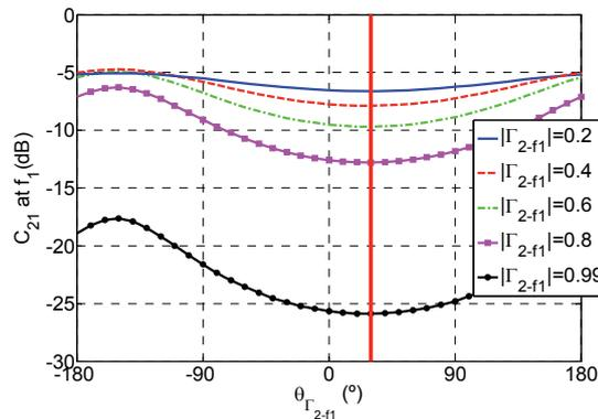
Fig. 8. Variation of coupling with  $\theta_{\Gamma_2^{f_1}}$  for dual band two-port small antenna at  $f_1=950$  MHz for different values of  $|\Gamma_2^{f_1}|$ .
