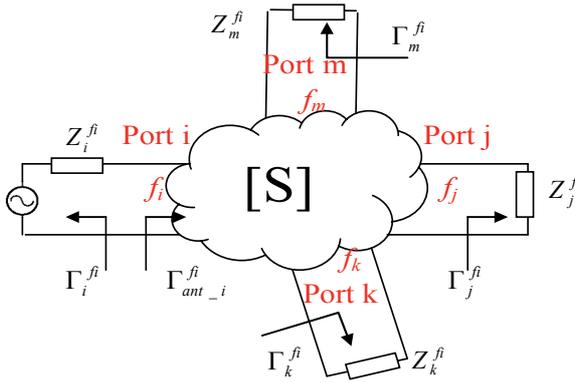
Fig. 1. Multipoint multiband antenna model.
