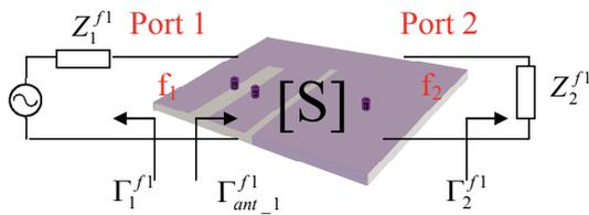
Fig. 6. Two-port dual band antenna model.
