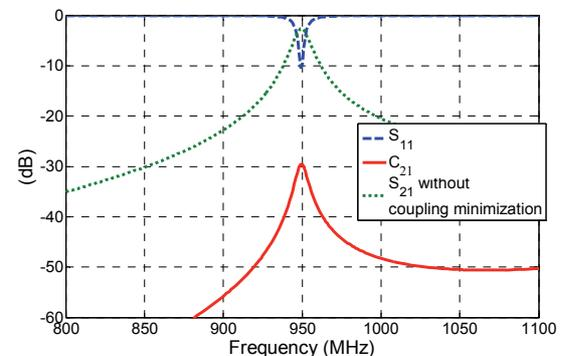
Fig. 13. Two-port dual band small antenna optimized for minimum coupling. Results for 950 MHz.
