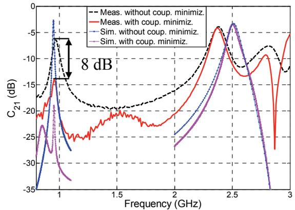
Fig. 10. Coupling improvement at  $f_1 = 950\text{ MHz}$ .
