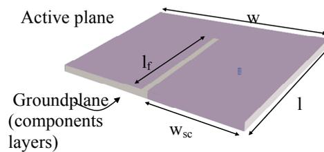
Fig. 3. 950 MHz antenna design.
