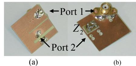
Fig. 12. Two port dual band small antenna prototype. (a) Active layer. (b) Bottom layer with 2 element load  $Z_2^{f_1, f_2}$  at port 2 and SMA connector at port 1.
