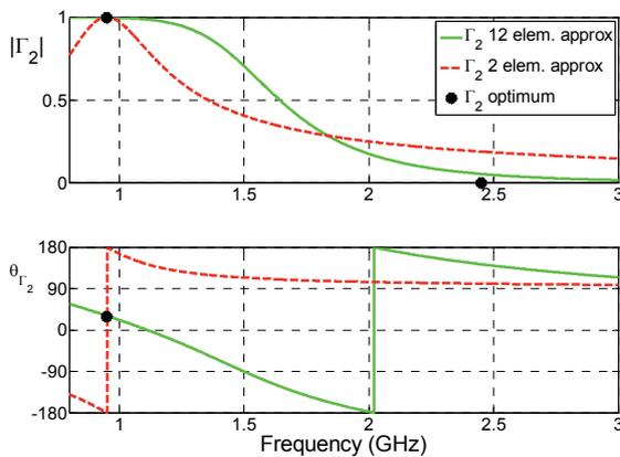
Fig. 9. Solutions for the optimum load for minimum coupling.
