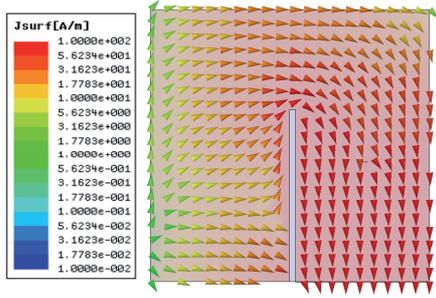
Fig. 4. Surface density current for the one-port patch antenna.
