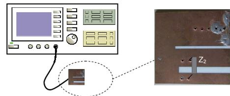
Fig. 11. Coupling characterization setup.
