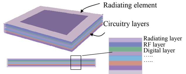
Fig. 2. Node integrated architecture.
