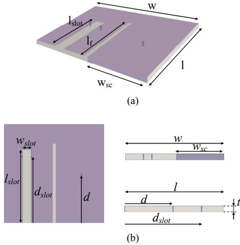
Fig. 5. Two-port dual band small antenna: (a) 3D view, (b) top and lateral views.
