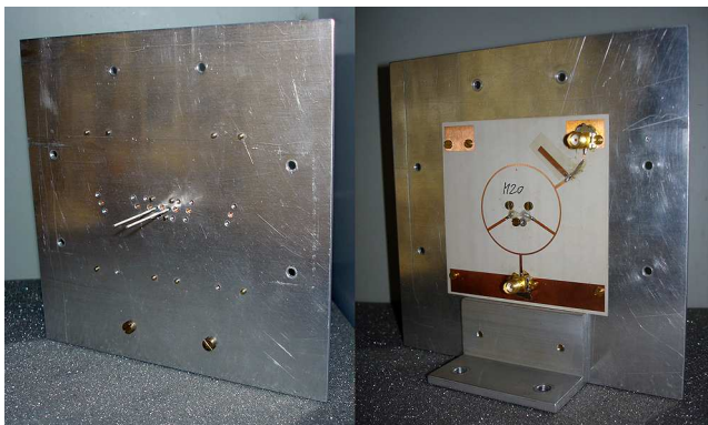
Fig. 6. Two-element monopole array with a radiator separation of \lambda/20 at 2.45 GHz. The right-hand side photograph shows the hybrid-coupler based decoupling and matching network mounted to the rear of the ground plane.
