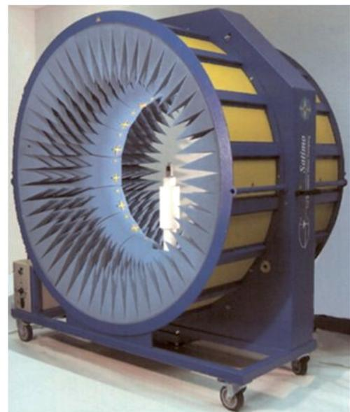
Fig. 1. StarLab: 800MHz to 18GHz Spherical Near Field Antenna Measurements System.
