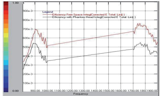
Fig. 19. Efficiency Measurements – Free-space (red curve), talk position (black curve)
