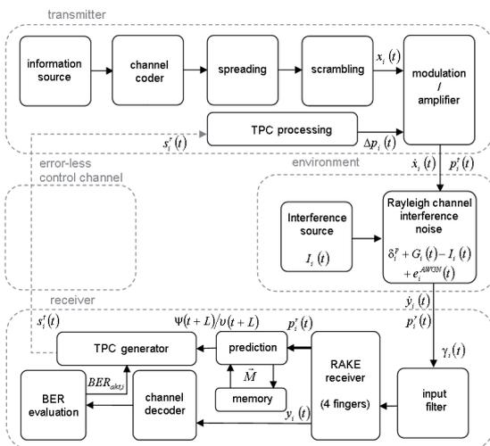
Fig. 4. WCDMA based transmitter/receiver block diagram.
