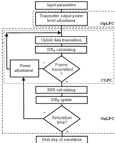
Fig. 1. Basic link adaptation algorithm.
