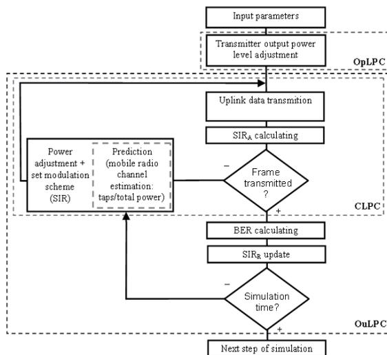
Fig. 2. Predictor based link adaptation algorithm.
