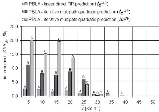
Fig. 6. Reduction of  $BER_{akt}$  for simulated PBLA algorithms.
