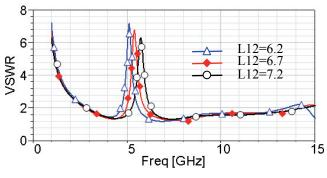
Fig. 5. Simulated VSWR for various L12 in mm with R1 = 4.9 mm and R2 = 4.6 mm.
