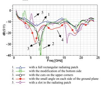
Fig. 3. Simulated reflection coefficient for different shapes of the radiation patch and the ground plane.
