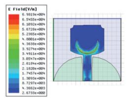
Fig. 8. Simulated current distribution of the antenna at 5.5 GHz.
