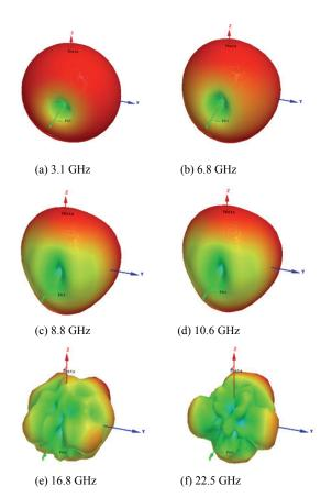
Fig. 7. Simulated radiation patterns at specific frequencies.
