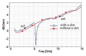
Fig. 9. Simulated gain of the antenna without and with a slot.
