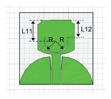
Fig. 4. Geometry of the antenna with a C-shaped slot, R1 = 4.9 mm, R2 = 4.6 mm, L11 = 8 mm, L12 = 6.7 mm.
