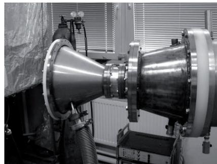
Fig. 14. View of fabricated axial vircator connected to the pulse forming line.
