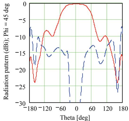
**Fig. 6.** Radiation pattern of the two-layer antenna in  $\varphi = 45^\circ$ -plane (bold – co-polar, dashed – cross-polar),  $f_0 = 11.72$  GHz.
