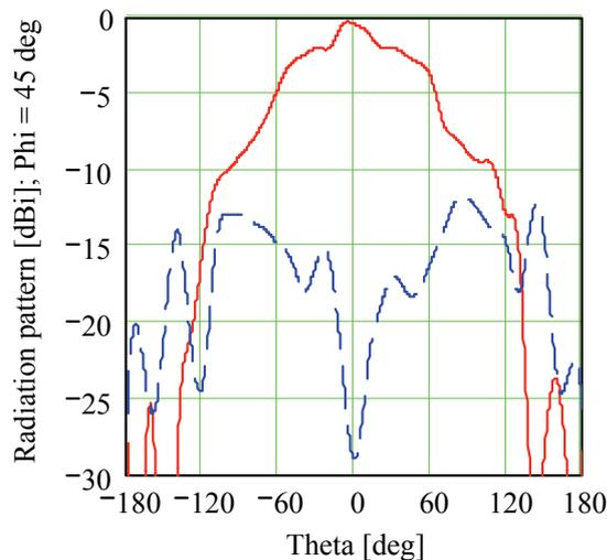
Fig. 8. Radiation pattern of the antenna with a screen in  $\varphi = 45^\circ$ -plane (bold – co-polar, dashed – cross-polar),  $f_0 = 12.01$  GHz.
