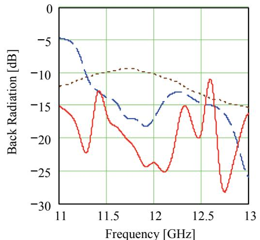
Fig. 4. Back Radiation BR versus frequency of the three antenna models (dotted – two-layer antenna, dashed – antenna with a reflector, bold – antenna with a screen).
