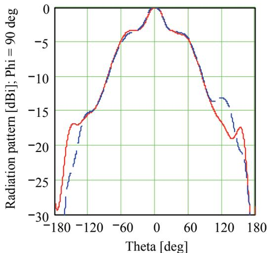
Fig. 9. Radiation pattern of the antenna with a screen in  $\varphi = 90^\circ$ -plane (bold – CST Microwave Studio 5, dashed – HFSS 10),  $f_0 = 12.01$  GHz.
