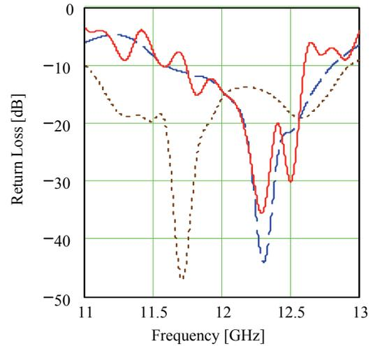
Fig. 2. Return Loss versus frequency of the three antenna models (dotted – two-layer antenna, dashed – antenna with a reflector, bold – antenna with a screen).
