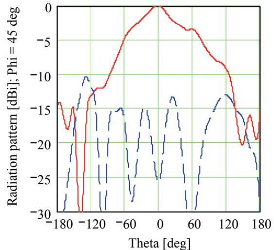
**Fig. 7.** Radiation pattern of the antenna with a reflector in  $\varphi = 45^\circ$ -plane (bold – co-polar, dashed – cross-polar),  $f_0 = 11.955$  GHz.
