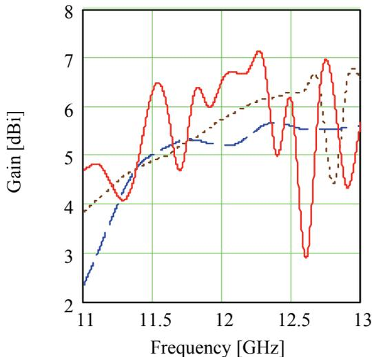
**Fig. 5.** Gain  $G$  versus frequency of the three antenna models (dotted – two-layer antenna, dashed – antenna with a reflector, bold – antenna with a screen).
