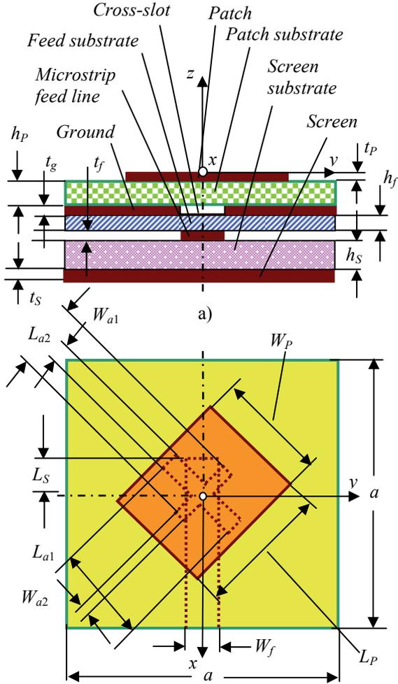
Fig. 1. Geometry of the antenna with a screen: (a) cross section, (b) front view.
