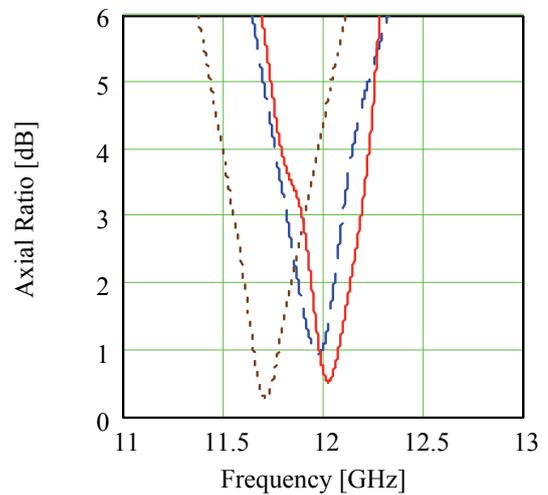
Fig. 3. Axial Ratio AR versus frequency of the three antenna models (dotted – two-layer antenna, dashed – antenna with a reflector, bold – antenna with a screen).
