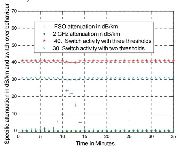
Fig. 7. Rain event of May 2002 and behavior of wireless sensor network for selecting communication link [35].
