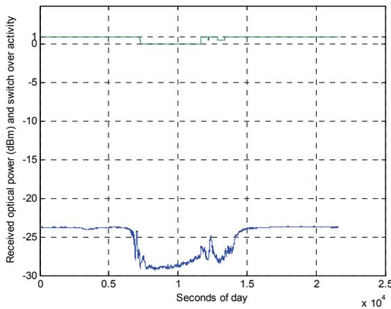
Fig. 2. Fog event of 22-11-2005 and behavior of wireless sensor network for selecting communication link.
