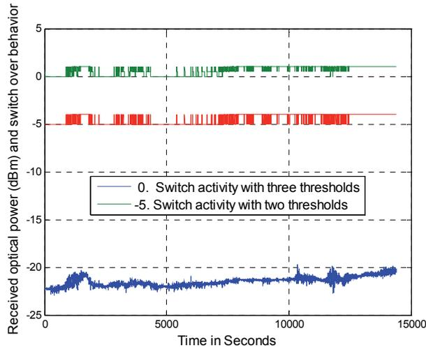
Fig. 5. Snow event of 02-02-2009 and behavior of wireless sensor network for selecting communication link [35].
