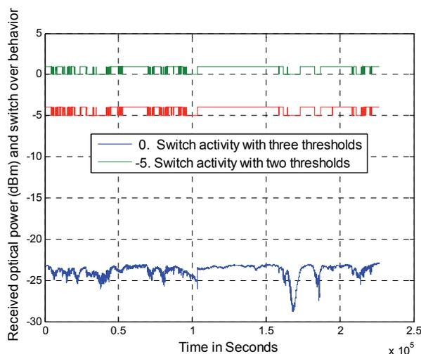
Fig. 6. Snow event of 28-11-2005 and behavior of wireless sensor network for selecting communication link [35].
