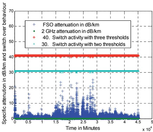
Fig. 8. Rain event of the whole year of 2002 and behavior of wireless sensor network for selecting communication link [35].
