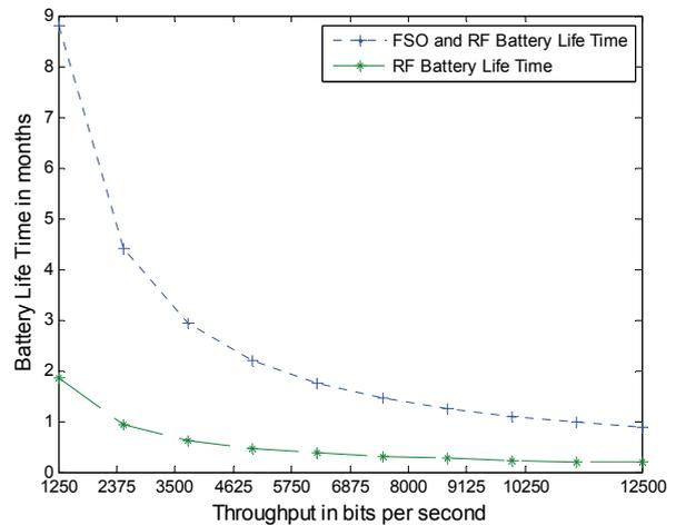
Fig. 11. 250 mAh battery life time for wireless sensor without microprocessor power consumption using RF only and both RF and FSO [35].
