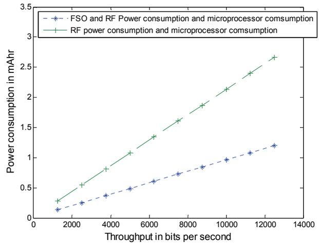
Fig. 10. Power consumption including microprocessor consumption for wireless sensor using RF only and both RF and FSO.
