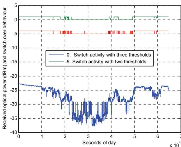
Fig. 3. Fog event of 31-01-2006 and behavior of wireless sensor network for selecting communication link.
