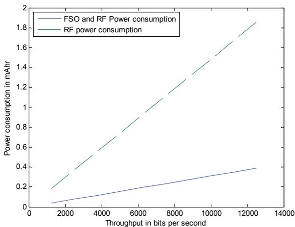
Fig. 9. Power consumption without microprocessor power consumption for wireless sensor using RF only and both RF and FSO [35].
