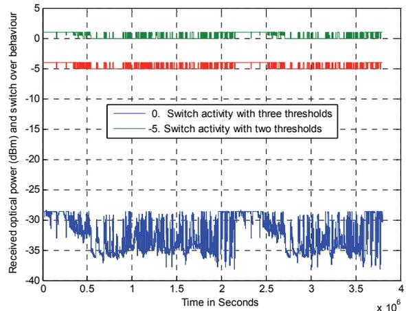
Fig. 4. All recorded fog events and behavior of wireless sensor network for selecting communication link.
