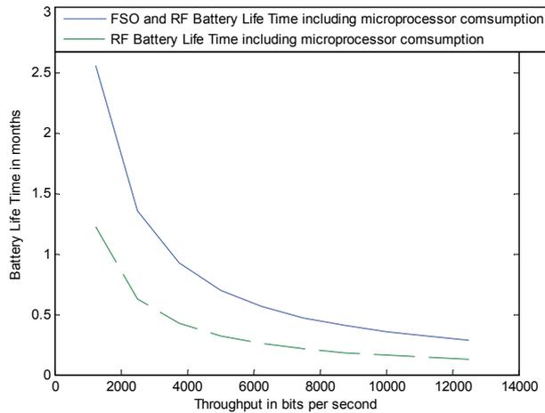
Fig. 12. 250 mAh battery life time including microprocessor power consumption for wireless sensor using RF only and both RF and FSO.
