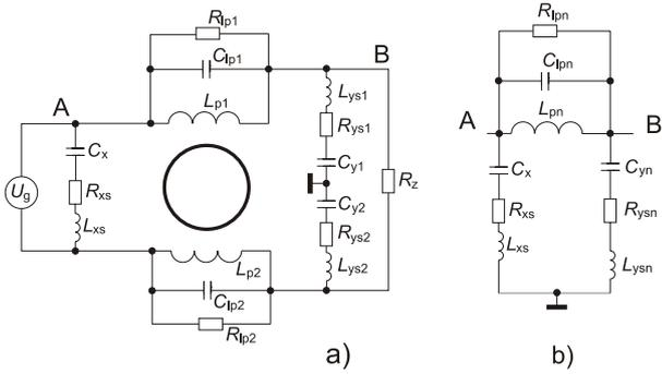
Fig. 5. Real model of Schurter 5110.1033.1 filter in symmetrical system a), reduced equivalent model in symmetrical system b).
