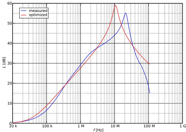
**Fig. 10.** Comparison of measurement characteristic and optimized characteristic of the Schurter 5110.1033.1 filter in asymmetrical measuring system.
