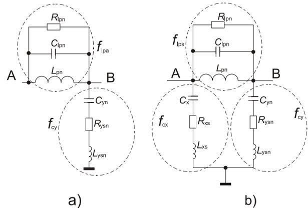
Fig. 7. The reduced equivalent circuits for the asymmetric a) and symmetric b) measuring systems.
