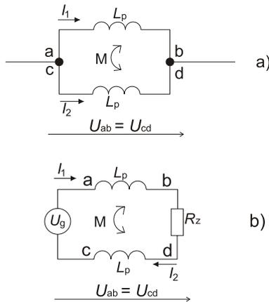
Fig. 6. The connection of the current compensated inductor in asymmetrical system a) and in the symmetrical system b).
