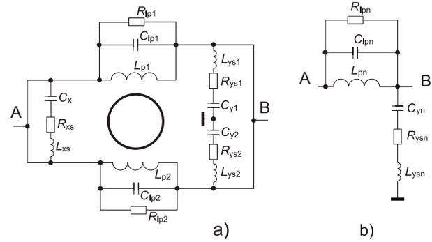
Fig. 4. Real model of Schurter 5110.1033.1 filter in asymmetrical system a); reduced equivalent model in asymmetrical system b).
