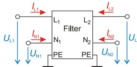
Fig. 3. The EMI filter as a six-pole.
