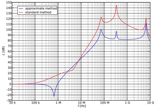
**Fig. 9.** Simulation of the insertion loss of the Schurter 5110.1033.1 filter in the symmetrical measuring system for different impedance conditions.
