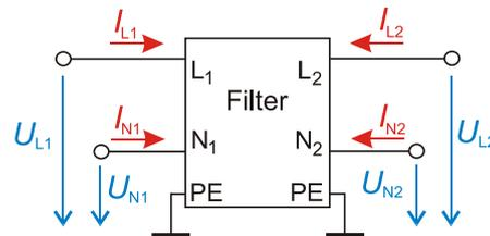
Fig. 3. The EMI filter as a six-pole.
