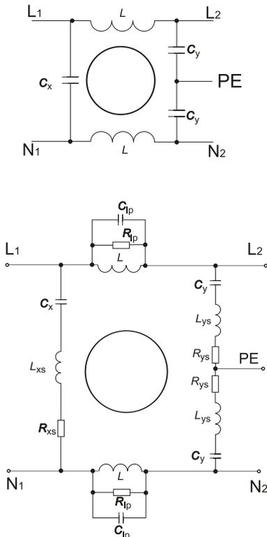
Fig. 2. Basic model of the Schurter 5110.1033.1 filter and its enlarged circuitry.
