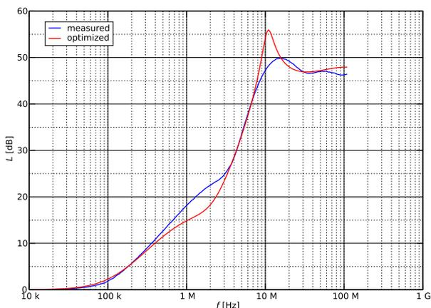
**Fig. 11.** Comparison of measurement characteristic and optimized characteristic of the Schurter 5110.1033.1 filter in symmetrical measuring system.
