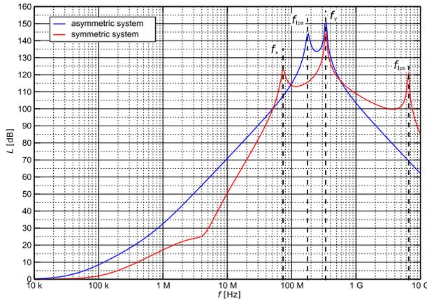
**Fig. 8.** Simulation of the insertion loss of the Schurter 5110.1033.1 filter in asymmetric and symmetric measuring systems.
