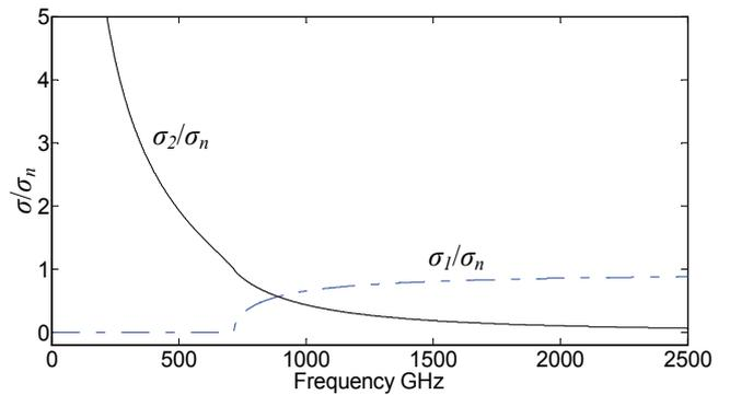
Fig. 6. The normalized complex conductivity of niobium at 4.2 K, computed using Mattis and Bardeen equation.
