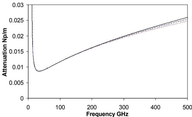
**Fig. 2.** Attenuation of TE<sub>11</sub> mode above cutoff. The solid line was calculated using our method, dotted line using Stratton's method, and the dashed line using the perturbation method.
