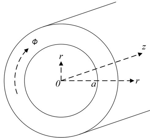
Fig. 1. A circular waveguide.
