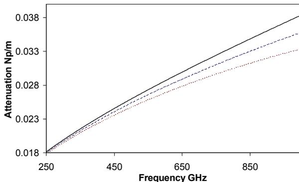
Fig. 4. Attenuation of TE<sub>11</sub> mode at millimetre wave frequencies. The solid line was calculated using our method, dotted line using Stratton's method, and the dashed line using the perturbation method.
