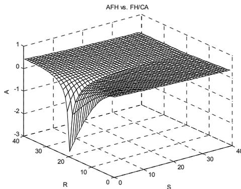
Fig. 7. Comparing the performance of system FH/CA with AFH in a band with static and dynamic jammers ( $N = 100$ ,  $R_{MAX} = 20$ ,  $G = 2$ ,  $R = 1$  to 40 and  $S = 1$  to 40).
