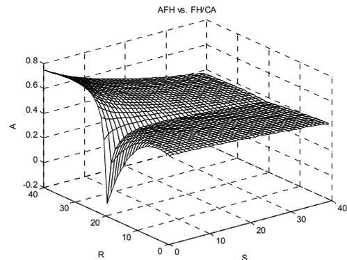
Fig. 8. Comparing the performance of system FH/CA with AFH in a band with static and dynamic jammers ( $N = 100$ ,  $R_{MAX} = 20$ ,  $G = 3$ ,  $R = 1$  to 40 and  $S = 1$  to 40).
