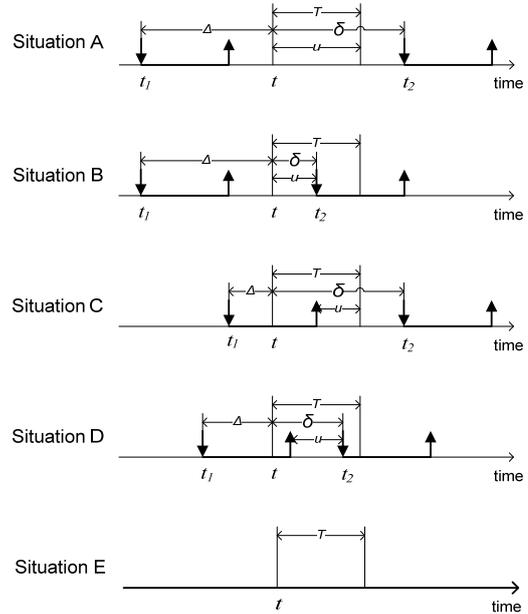
Fig. 1. Possible situations in occupying channels by FH/CA station.
