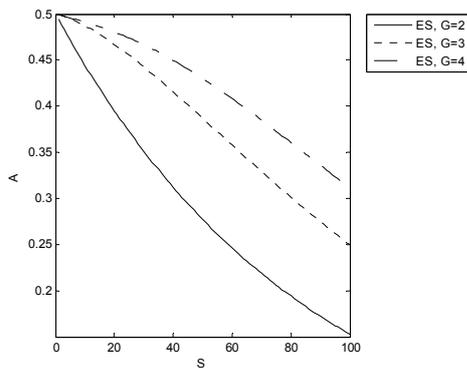
Fig. 6. Comparing the performance of system FH/CA with AFH in a band with dynamic jammers ( $N = 100$ ,  $G = 2, 3$  and  $4$ ,  $R = 0$  and  $S = 1$  to 100).
