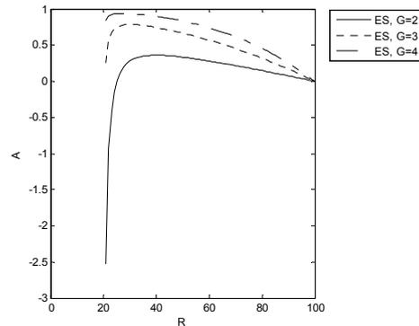
**Fig. 5.** Comparing the performance of system FH/CA with AFH in a band with static jammers ( $N = 100$ ,  $R_{MAX} = 20$ ,  $G = 2, 3$  and  $4$ ,  $R = 1$  to  $100$  and  $S = 0$ ).
