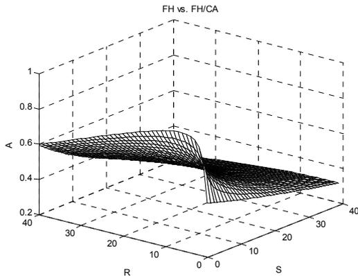
**Fig. 4.** Comparing the performance of system FH/CA with FH in a band with static and dynamic jammers ( $N = 100$ ,  $G = 2$ ,  $R = 1$  to  $40$  and  $S = 1$  to  $40$ ).
