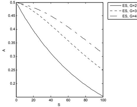
**Fig. 3.** Comparing the performance of system FH/CA with FH in a band with dynamic jammers ( $N = 100$ ,  $G = 2, 3$  and  $4$ ,  $R = 0$  and  $S = 1$  to  $100$ ).
