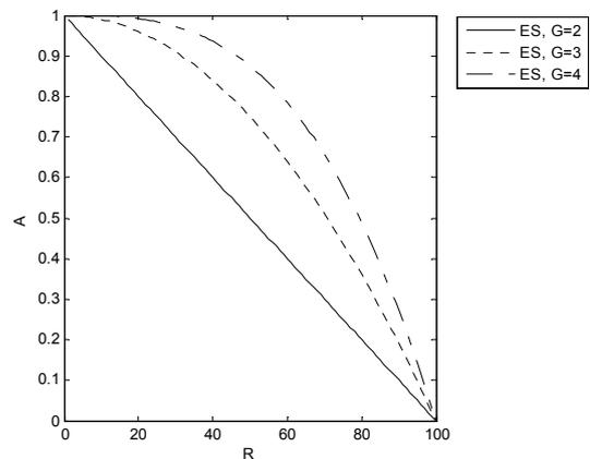
Fig. 2. Comparing the performance of system FH/CA with FH in a band with static jammers ( $N = 100, G = 2, 3$  and  $4, R = 1$  to  $100$  and  $S = 0$ ).
