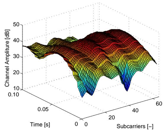
Fig. 3. Interpolated CSI matrix, method: Nearest.
