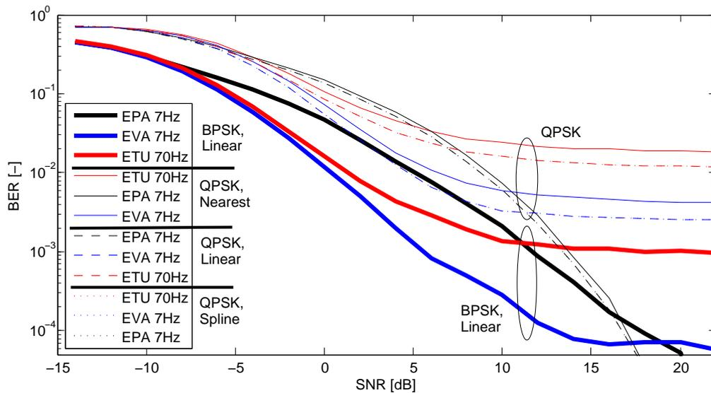
Fig. 4. The comparison of BER performance for different interpolations methods for CSI estimation, different channel models and BPSK and QPSK inner modulation VSF-OFCDM.
