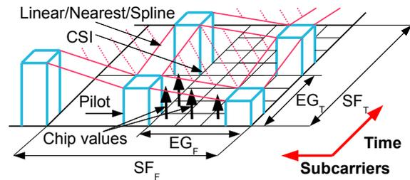
Fig. 1. Pilot insertion.
