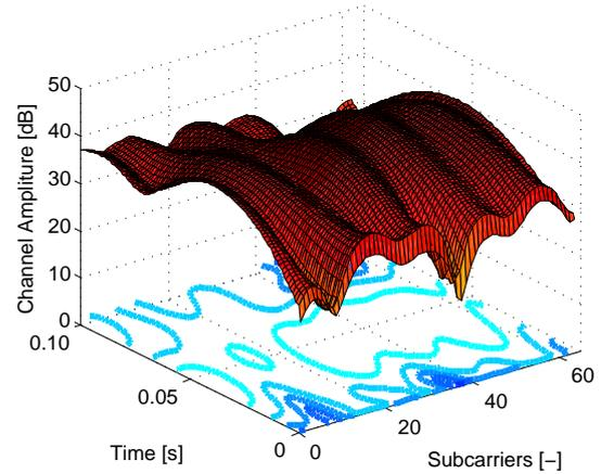
Fig. 2. Real CSI matrix (perfect knowledge of the channel state).
