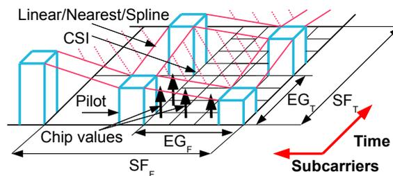
Fig. 1. Pilot insertion.
