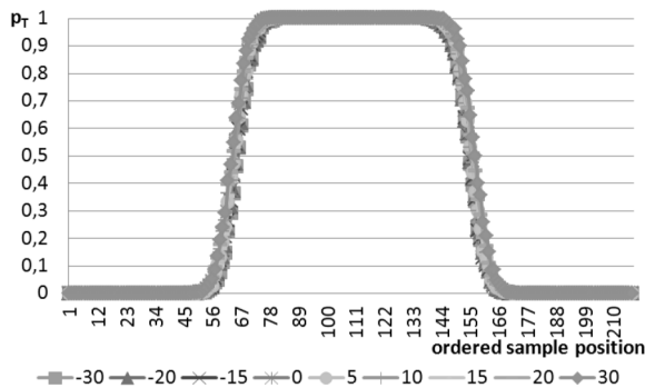
Fig. 6. Probability chart for samples of a jitter influenced clock signal CLJ accumulated during N = 1000 of T_Q periods for PLL-TRNG with PLL Configuration B with K_D = 217 for temperatures in range T = (-30^\circ\text{C}, +30^\circ\text{C}) .
