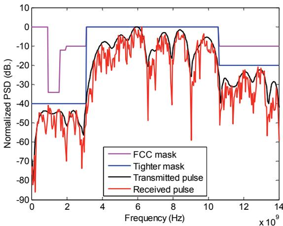
**Fig. 2.** The transmitted power spectrum of the UWB waveform designed by (14) and the corresponding power spectrum after RF effects and channel effect.
