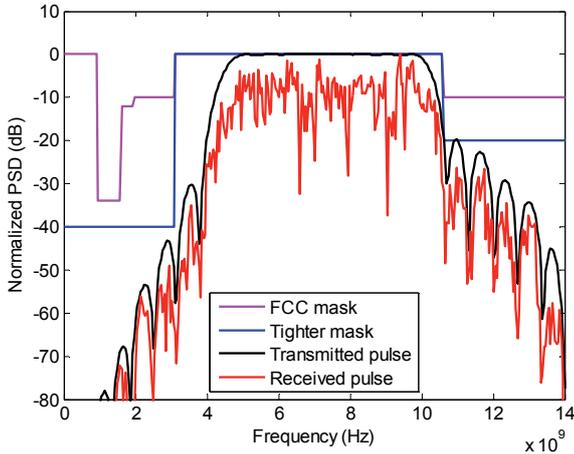
**Fig. 1.** The transmitted power spectrum of the UWB waveform designed by (10) and the corresponding power spectrum after RF effects and channel effect.
