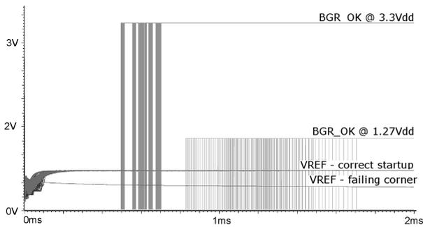
Fig. 8. Startup and BGR OK signal generation in all simulation corners.
