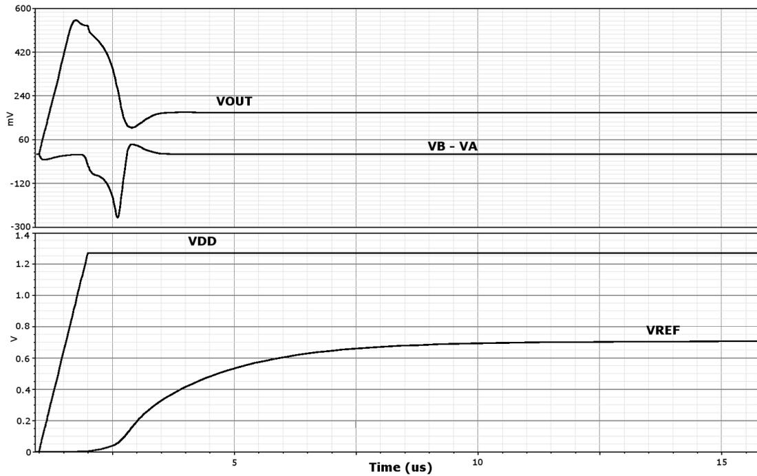
Fig. 7. Startup of the complete circuit in the typical technology corner. VDD curve shows ramped supply voltage simulating the real power supply. VOUT displays the voltage at the output of the OPAMP. The second waveform shows the differential voltage (VB - VA). VREF shows the startup of the output voltage from zero to defined voltage.
