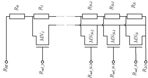
Fig. 6. The resistor ladder for trimming.
