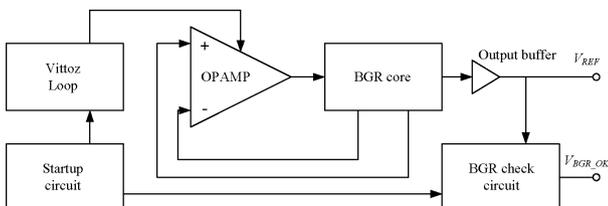
Fig. 2. Block schematic with external biased OPAMP selected.
