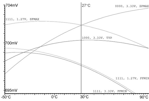
Fig. 9. Trimming range - temperature dependence.
