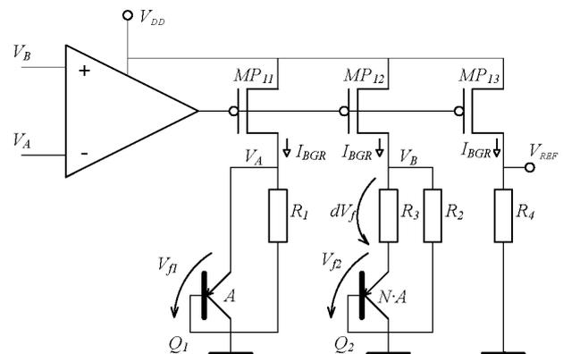
Fig. 1. BGR design according to H. Banba [1].
