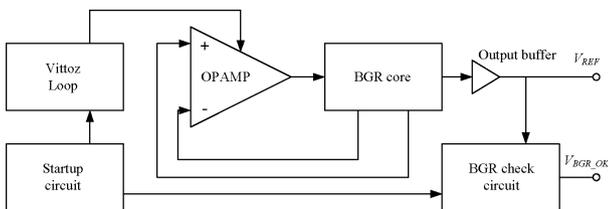
Fig. 2. Block schematic with external biased OPAMP selected.
