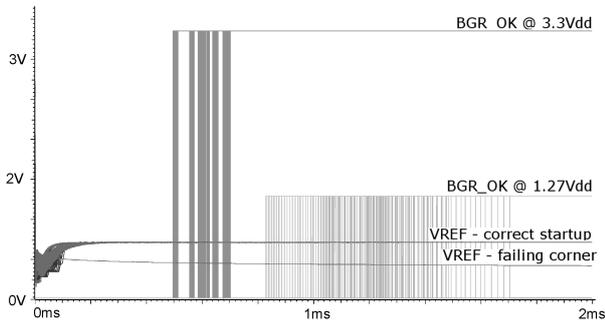
Fig. 8. Startup and BGR OK signal generation in all simulation corners.
