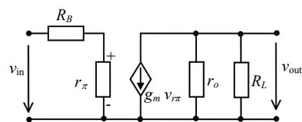
Fig. 1. AC model of simple amplifier with bipolar transistor.
