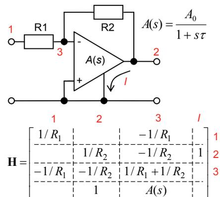
Fig. 4. Parametric simplification of an amplifier.
