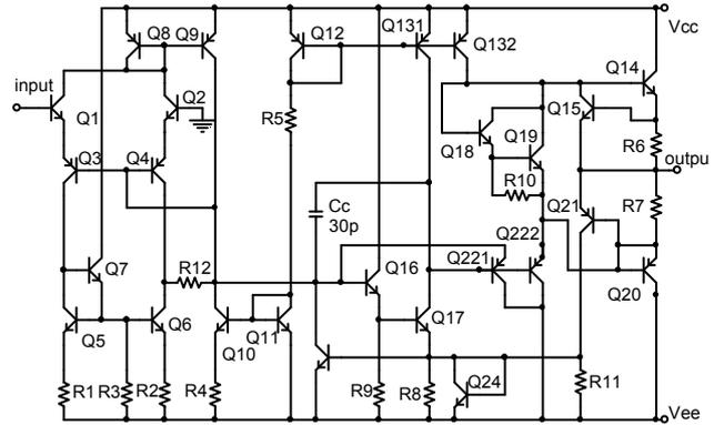
Fig. 9. Internal structure of  $\mu A741$ .
