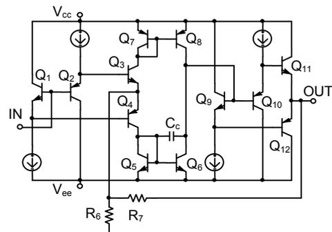
Fig. 10. Circuit with current-feedback amplifier (CFA).
