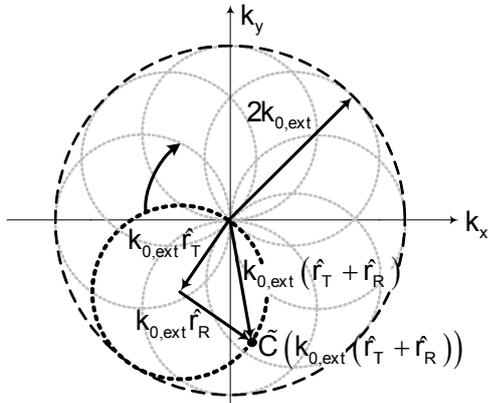
**Fig. 2.** 2D cut of the dielectric spectrum of the contrast. For a single transmitter and incidence frequency, the spectrum of the contrast is sampled on the surface of a sphere of radius  $k_{0,ext}$  centered at  $-k_{0,ext}\hat{r}_T$ . For another direction of incidence the sphere rotates.
