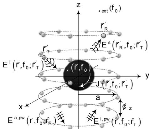
**Fig. 1.** The target of permittivity  $\epsilon(\vec{r}, f_0)$  is immersed in a medium of permittivity  $\epsilon_{ext}(f_0)$ . The measurement cylindrical array of antennas is composed by  $N_z$  rings of  $N_\phi$  antennas of radius  $a$ , separated a distance  $\Delta_z$ .  $\vec{r}'_{T,R}$  refers to the position of the transmitting and receiving antennas respectively, and  $\hat{r}'_{T,R}$  is the direction of the synthesized plane wave.
