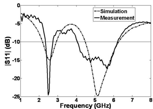
Fig. 3. Comparison of the simulated and measured return loss ( $|S_{11}|$ ) of the proposed 9-shaped monopole antenna for RFID and WLAN application.
