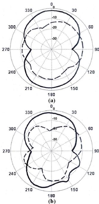
Fig. 5. Measured E-plane (Co-pol(solid line) and Cross pol(dotted line)) radiation patterns at (a) 2.45 GHz and (b) 5.2 GHz.
