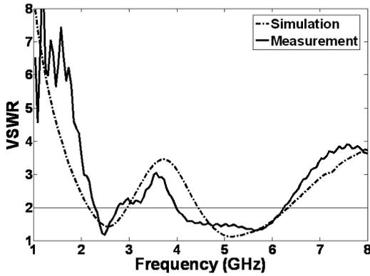
Fig. 4. Comparison of the simulated and measured VSWR of the proposed 9-shaped monopole antenna for RFID and WLAN application.
