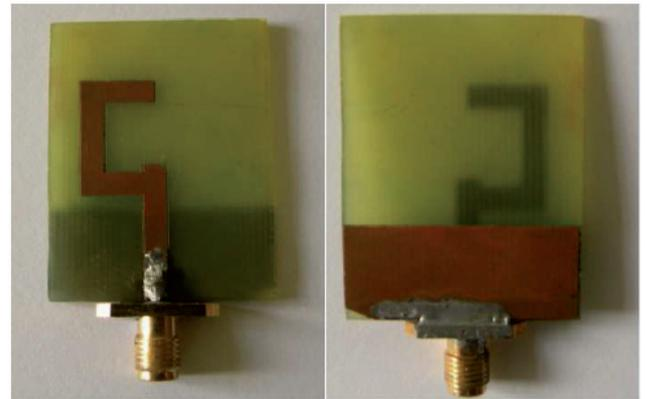
Fig. 2. Fabricated prototype of the 9-shaped monopole antenna for RFID and WLAN application. (a) Top View. (b) Bottom View.
