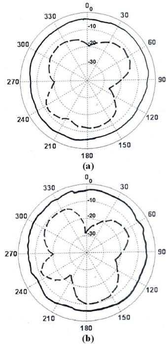
Fig. 6. Measured H-plane (Co-pol(solid line) and Cross pol(dotted line)) radiation patterns at (a) 2.45 GHz and (b) 5.2 GHz.
