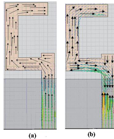
Fig. 7. Surface current distribution (A/m) of the proposed 9-shaped monopole antenna (a) at 2.45 GHz and (b) at 5.2 GHz.
